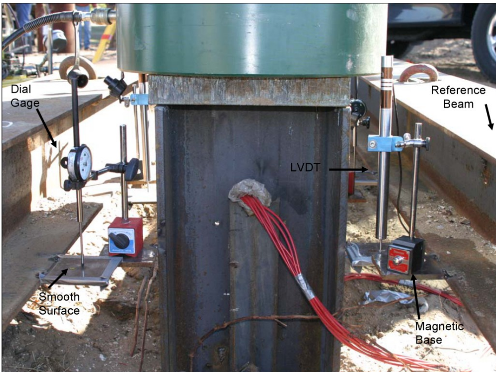
Figure 9-65. Load test movement monitoring components (FHWA, 2006a).
