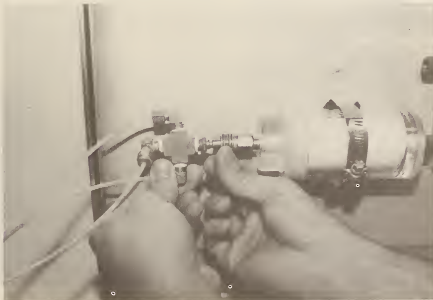
Fig. A-6. Connect return line manifold to desiccator.
