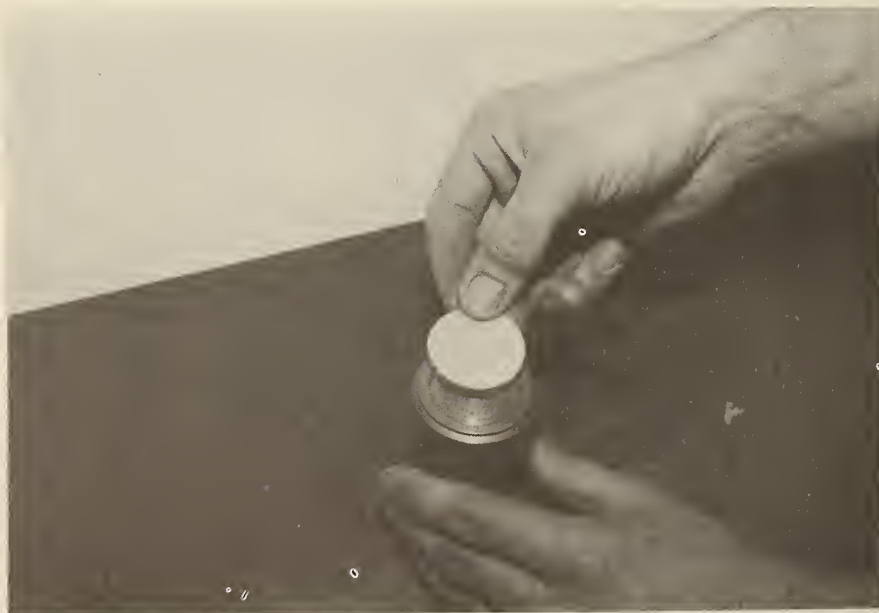
Fig. A-20. Disc is placed on a special forming die.
