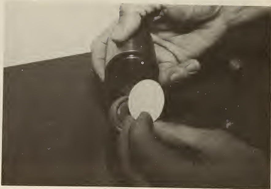
Fig. A-23. Disc, now cupped at the edge, is removed.
