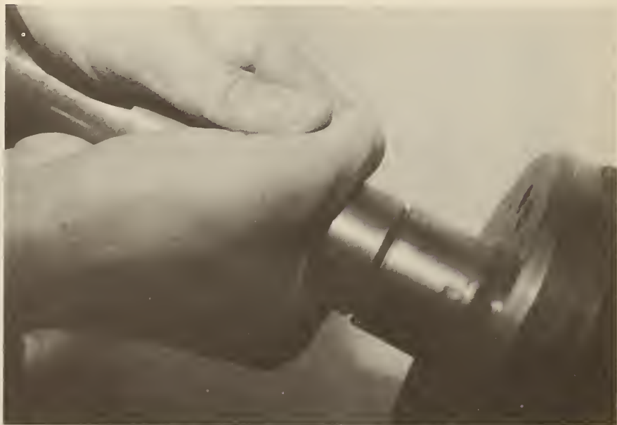
Fig. A-8. Vane is fastened to an special connector which allows drill rod weight to be lifted off the vane. Assembly is then attached to any conventional rotary exploration drilling machine.
