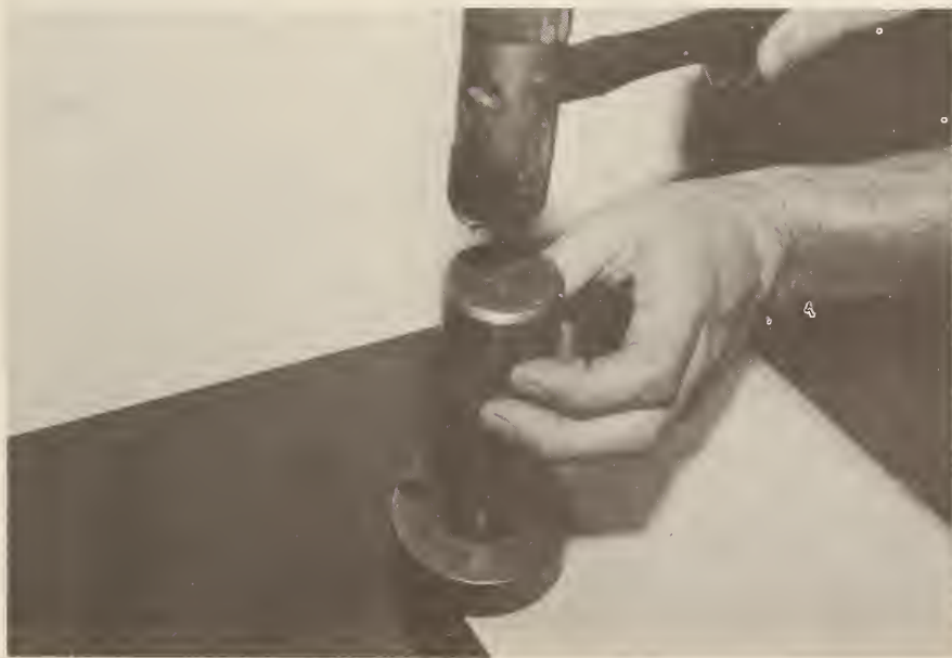
Fig. A-18. Punch is driven.
