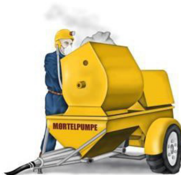
Figure 4.6 Grout pump (progressive cavity pump)
