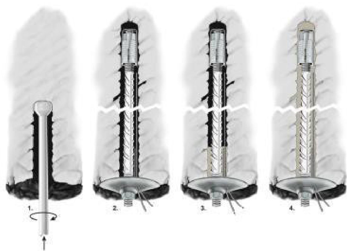
Figure 4.14 Installation of end-anchored and post-grouted bolt
