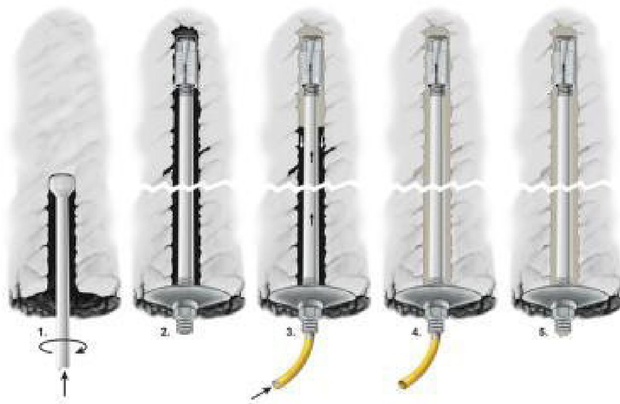
Figure 4.13 Installing a pipe bolt
