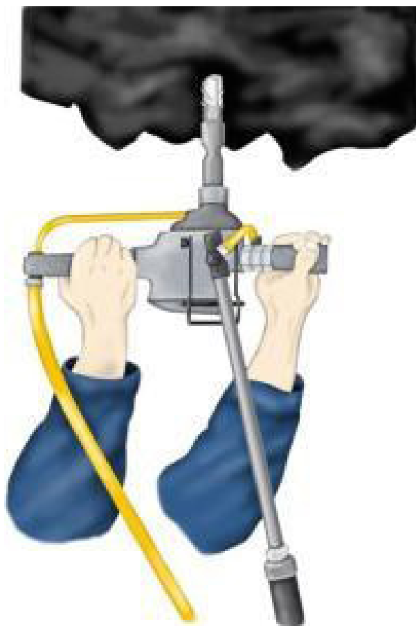
Figure 4.5 Pneumatic drill with feed column
