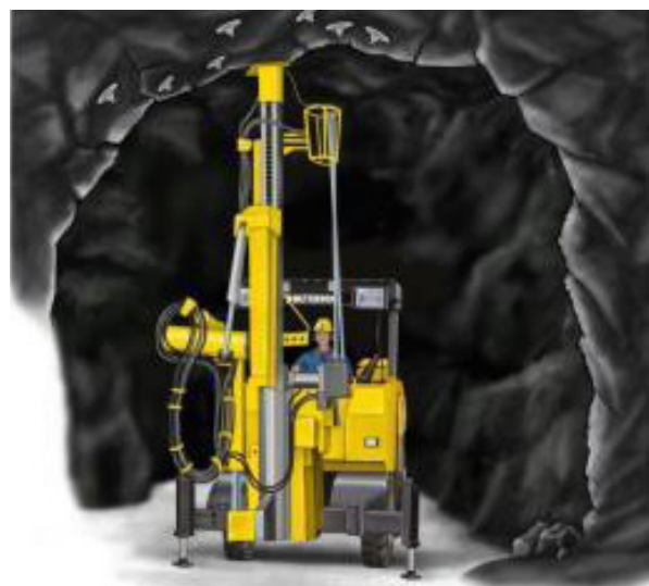
Figure 4.1 Fully mechanised bolting rig
