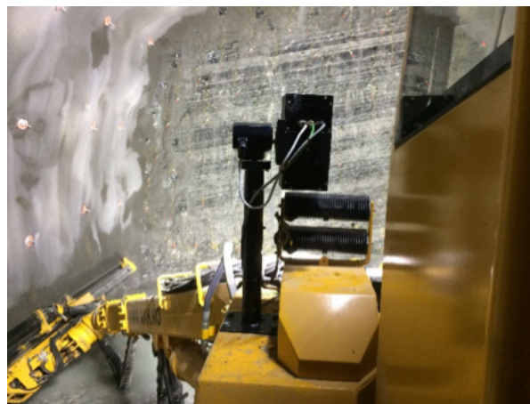
Figure 7.13. It can be documented using a handheld camera, in this case a tablet (left) or a fixed camera on a drilling or spraying rig (right).
