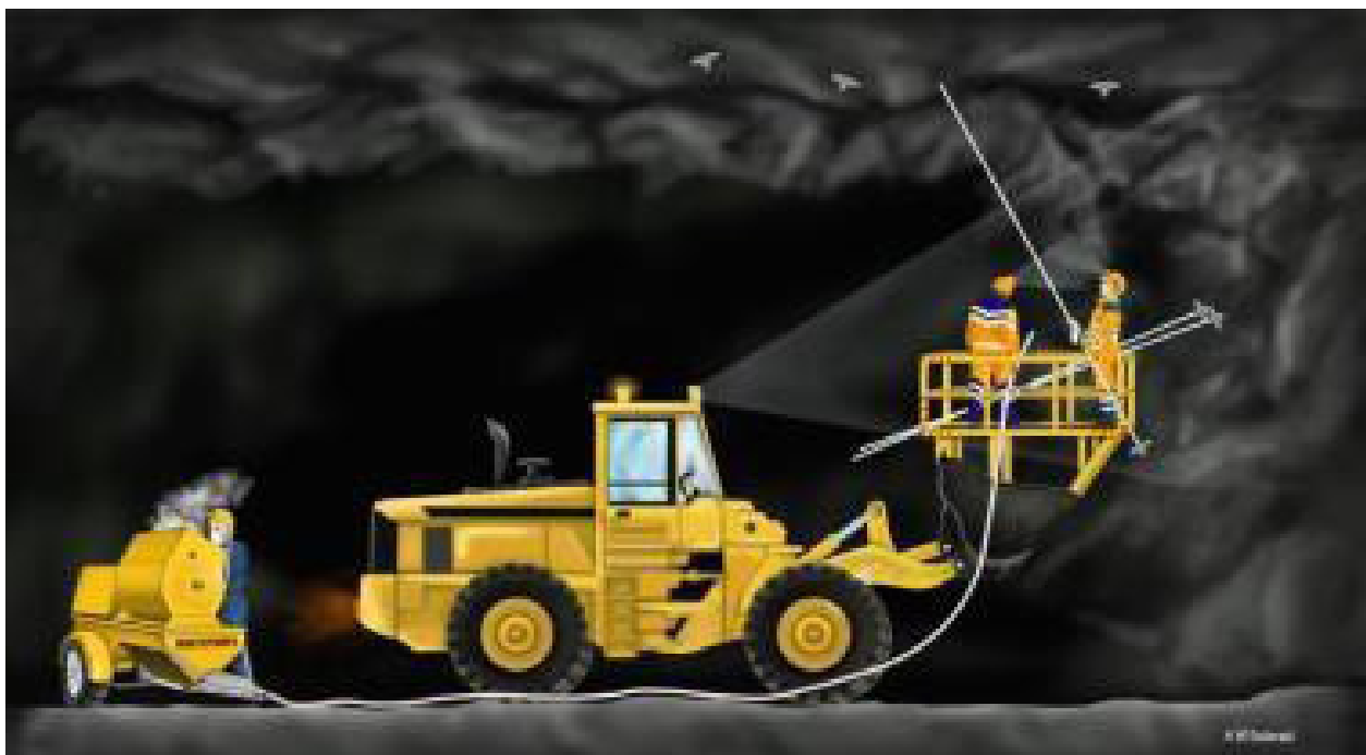
Figure 4.4 Wheel loader with basket
