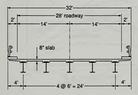
Figure 5.2: Typical Composite Girder Cross Sections Used in the Study of Differential-Settlement Effects.
