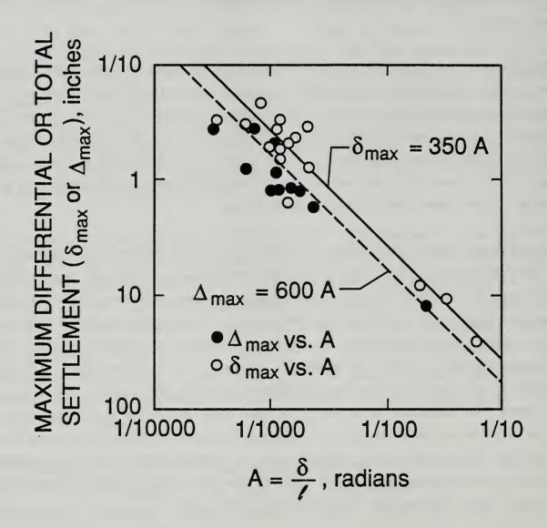
Figure 5.1: Correlations Between Total Settlements, Differential Settlements and Angular Distortions in Granular Soils (after Grant et al.,1974).
