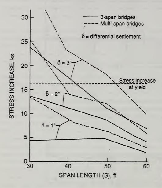
Figure 5.3: Stress Increases in Steel Girders of Typical Composite Girder Bridges Caused by Settlement Induced Negative Moments.
