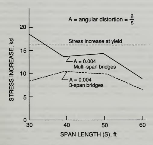
Figure 5.4: Stress Increases in Steel Girders of Typical Composite Girder Bridges Caused by Angular Distortions of 0.004 Radians.
