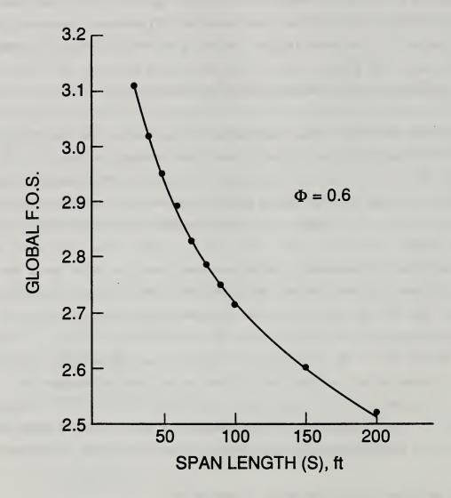
Figure 4.3 Correlation Between Span Length and Global Safety Factors Resulting from LRFD Design .
