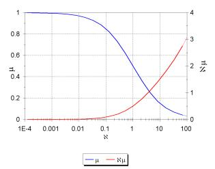
Figure 2. Softening Coefficient vs. Normalized Shear Strain (adapted in part from Vardanega and Bolton (2013))
