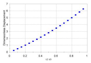
Figure 3. Dimensionless Displacement of Pile vs. Shear Stress Ratio
