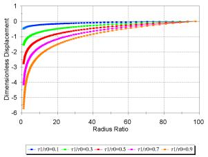
Figure 4. Soil Deflections as a Function of Radius Ratio
