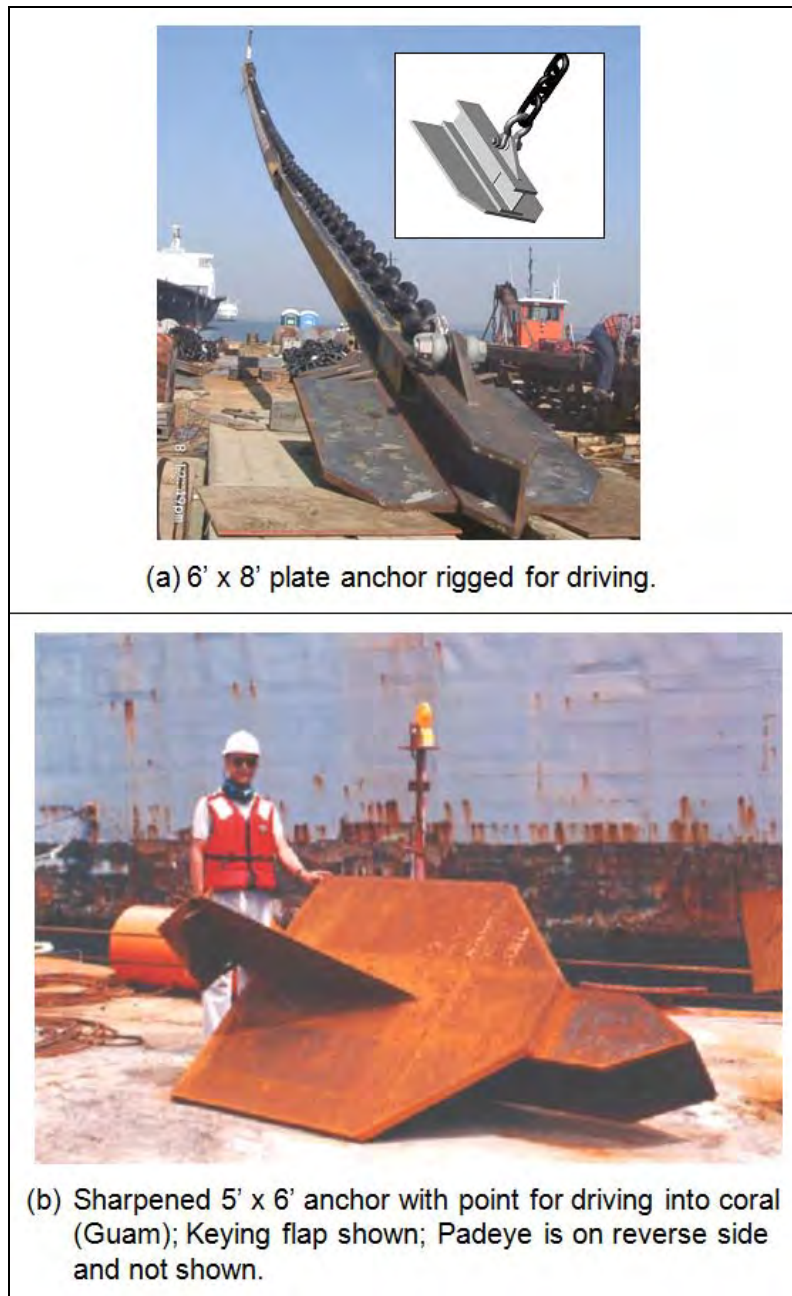
Figure 6.2-1. Sample impact/vibratory driven anchors.
