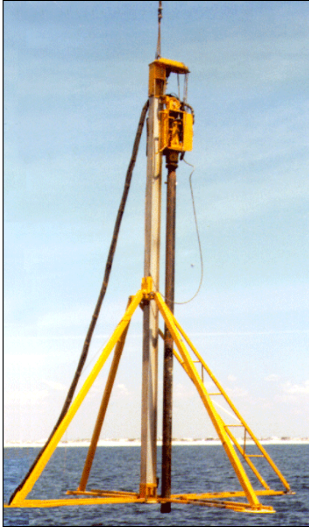
Figure 2.4-4. Alpine vibracore sampler (from Ref. 2-6).
