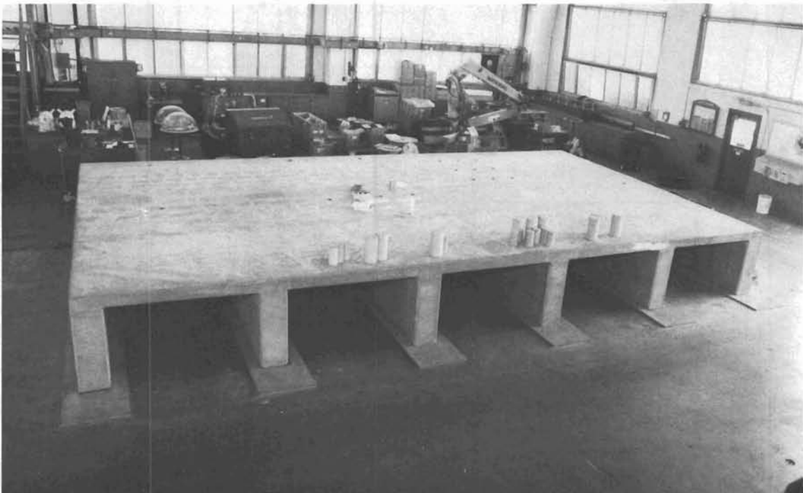
Figure 8. Completed pier deck scale model.
