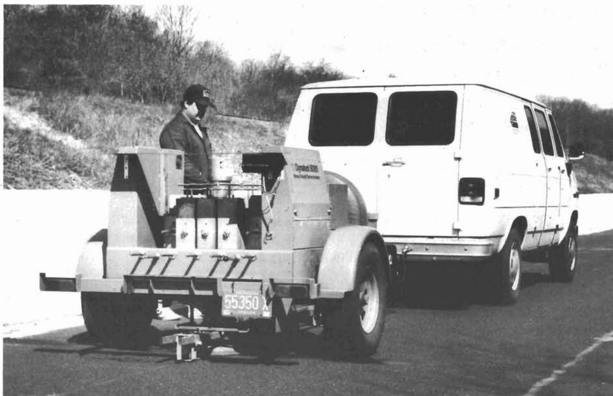
Figure 1 Falling weight deflectometer and tow vehicle.
