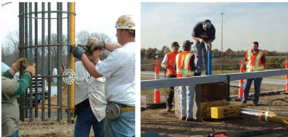
Figure 4-6: Measurement of lateral deformation in a test shaft using an inclinometer (from Brown et al. 2010).
