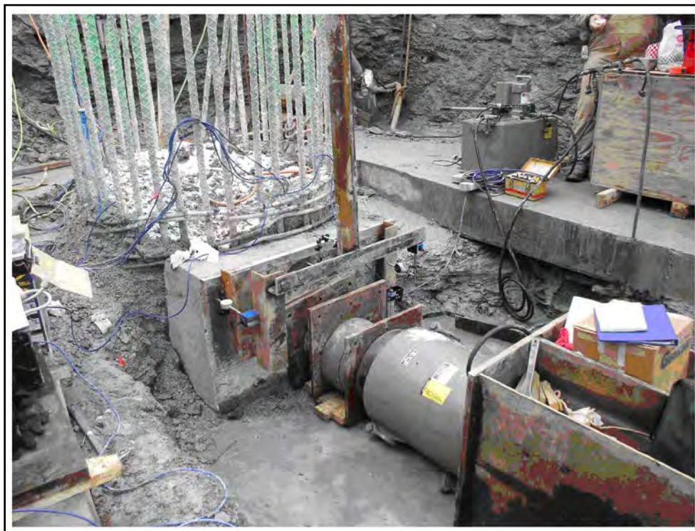
Figure 12-1: Example of a two-way lateral load test set-up for a drilled shaft.
