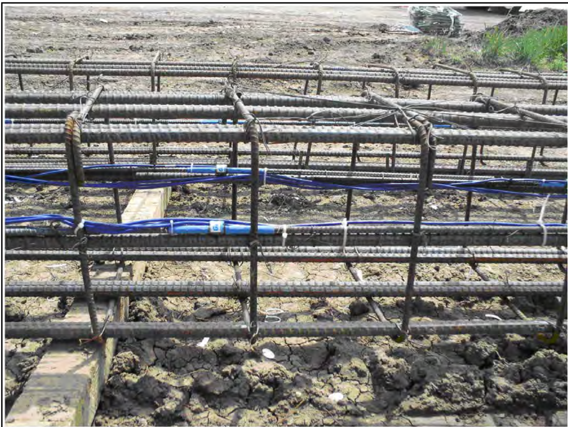
Figure 12-5: A pair of sister bar strain gauges attached to a reinforcement cage.
