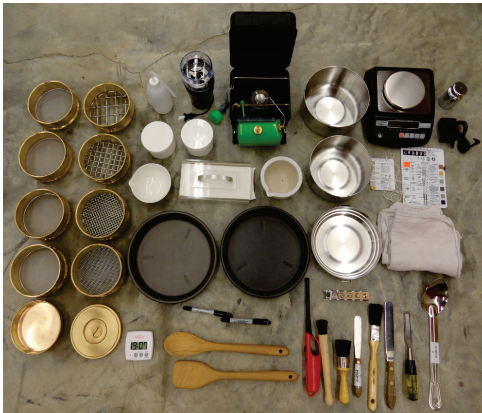
Figure 8. Wet-based Rapid Soils Analysis Kit as developed for the CALDERA program.
