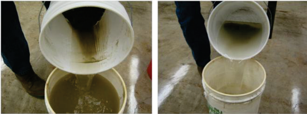
Figure 6. Wash and decanting process for removing fines (minus #200 sieve) material using the Cornell quick wash procedure.
