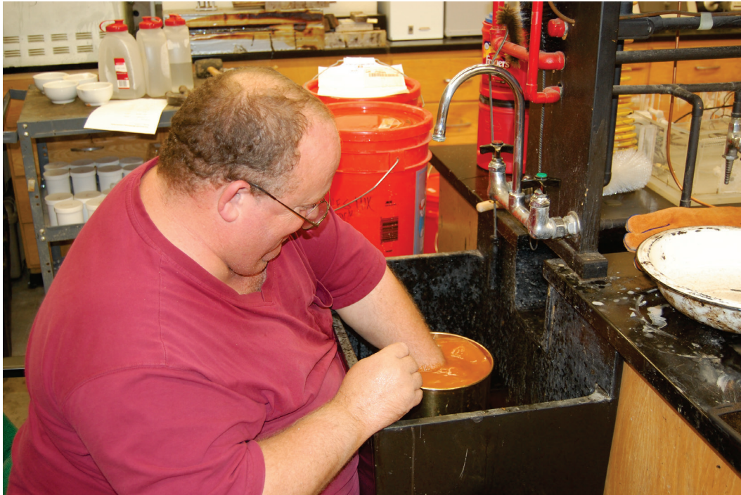
Figure 23. Washing fines in deep #200 sieve for ASTM procedure.
