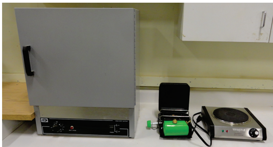
Figure 2. Army soils kit drying oven in comparison to RSAK drying apparatus.
