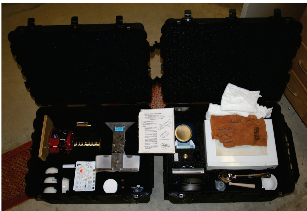
Figure 7. Dry-based Rapid Soils Analysis Kit (D-RSAK) as packaged for the JRAC program.
