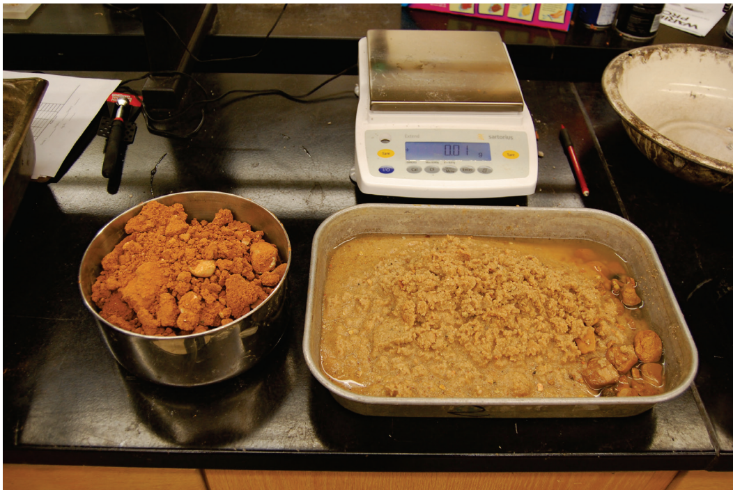
Figure 22. Clay gravel dried and after washing over #200 sieve (note large ASTM sample size used versus a typical 500-g RSAK sample).
