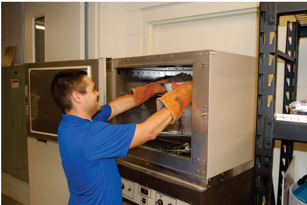
Figure 24. Oven drying limestone soil samples in large oven for at least 16 hr.
