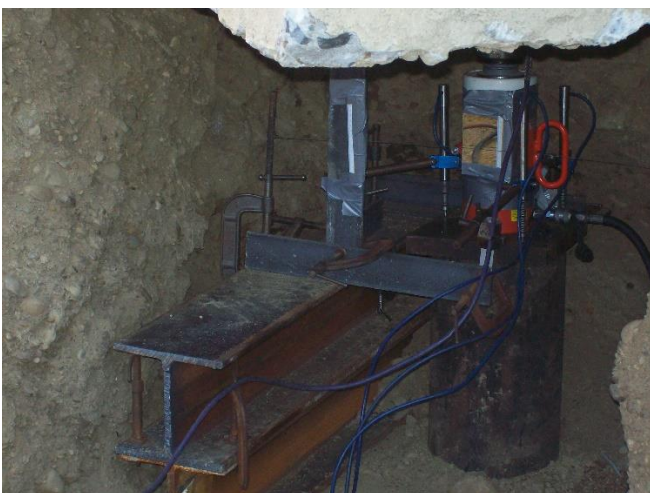
A. Load test setup for north abutment
