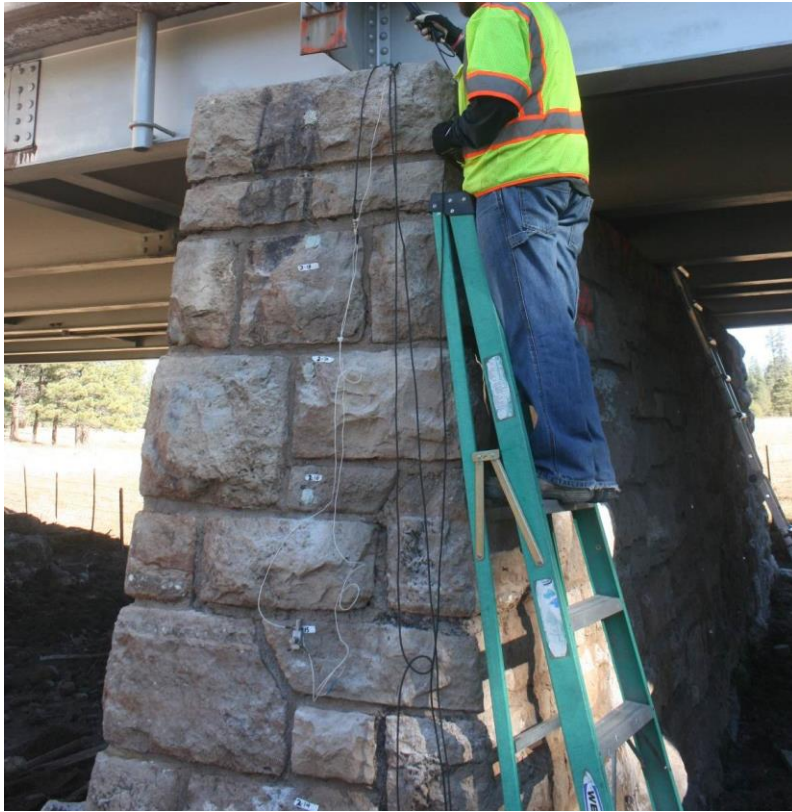
Figure 37. Photo. Performing ultraseismic testing on a pier
