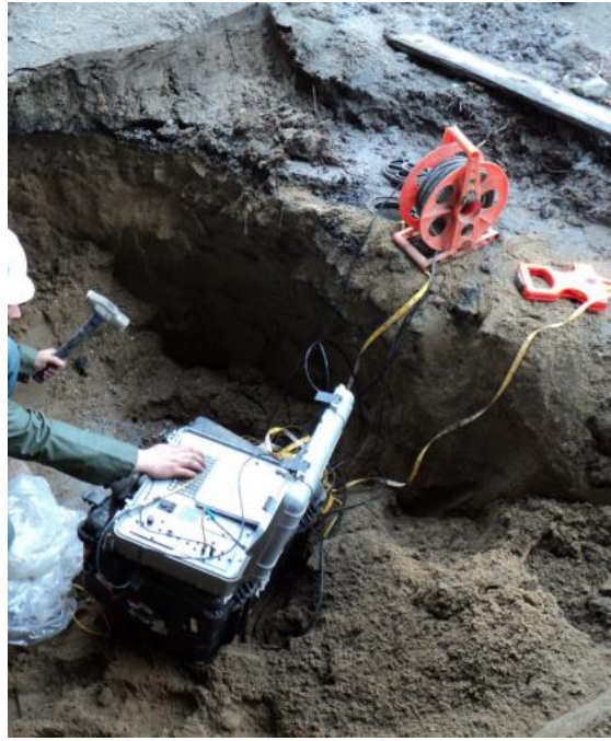
Figure 17. Photo. Parallel Seismic (PS) setup for abutment of U.S. Route 1 Bridge in Maine
