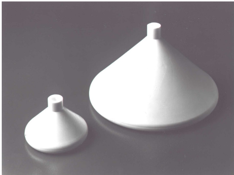
Figure 5-6. Plugs to Channel Forces into Stemming.
