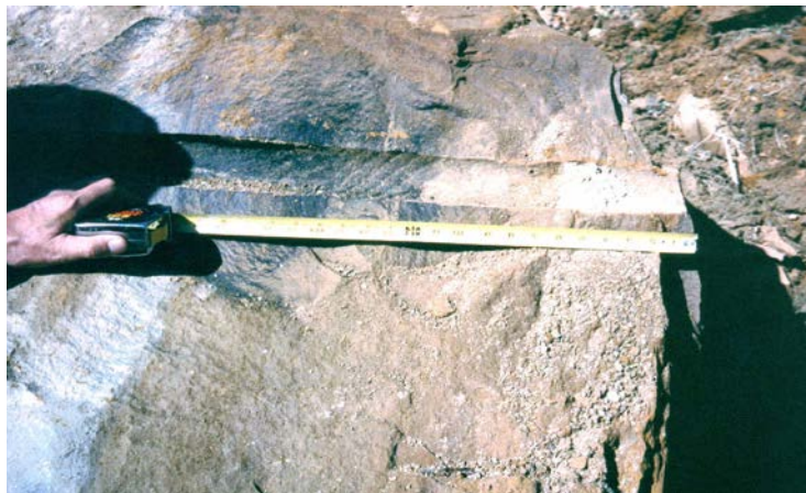
Figure 5-5. Stemming Material Compaction Immediately Above Charge in Borehole.
