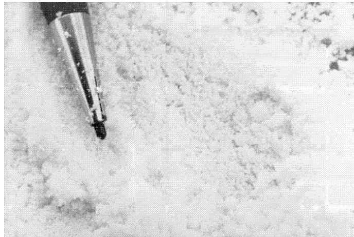
Figure 2-19. AN Prills after Temperature Cycling
