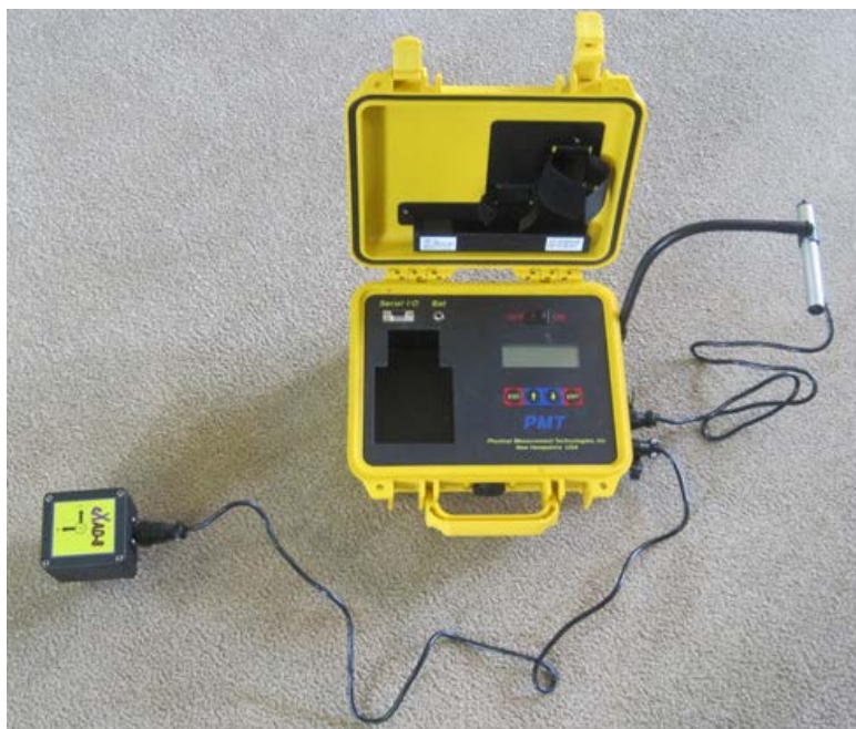
Figure 8-11. Seismograph with Attached Geophone.
