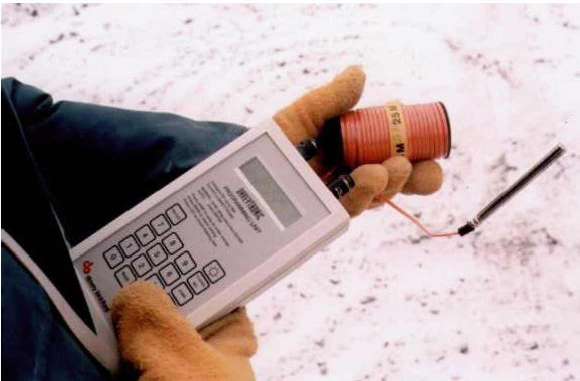
Figure 2-22. DavyFire Electronic Blasting Cap.
