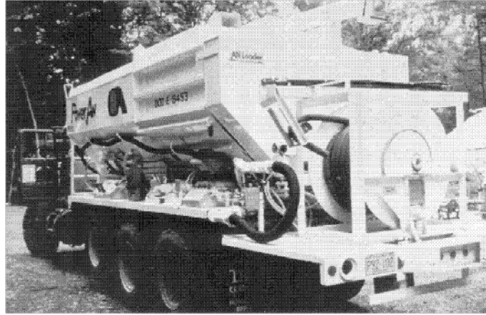
Figure 2-16. Heavy ANFO Bulk Loading Truck
