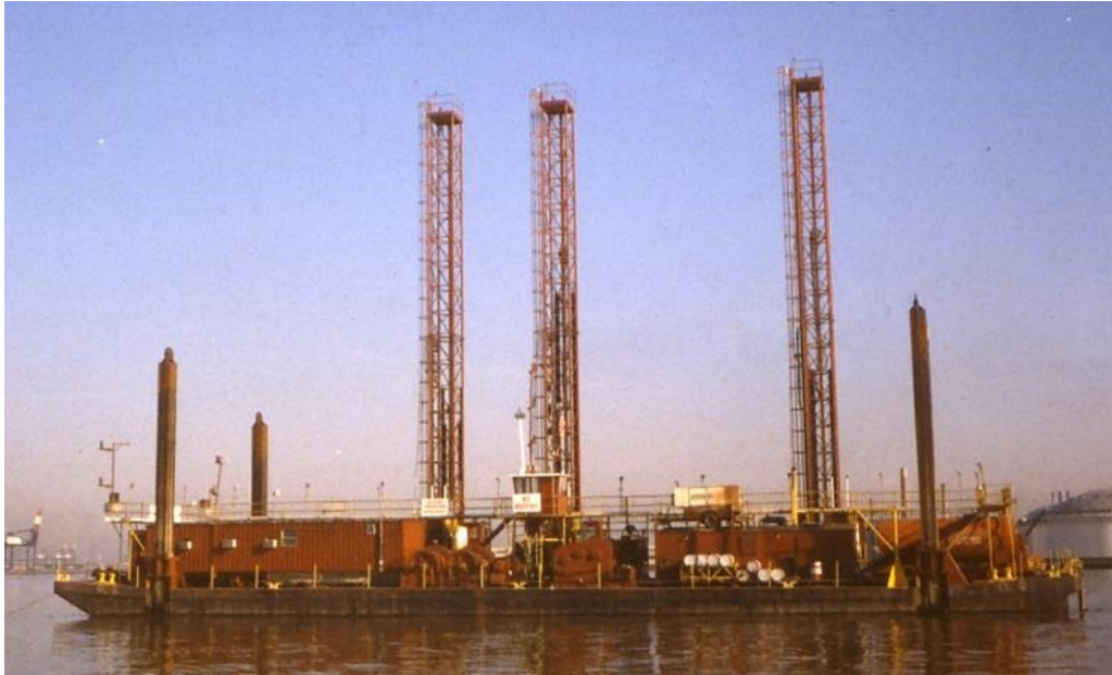
Figure 7-1. Photo of Drill Barge.
