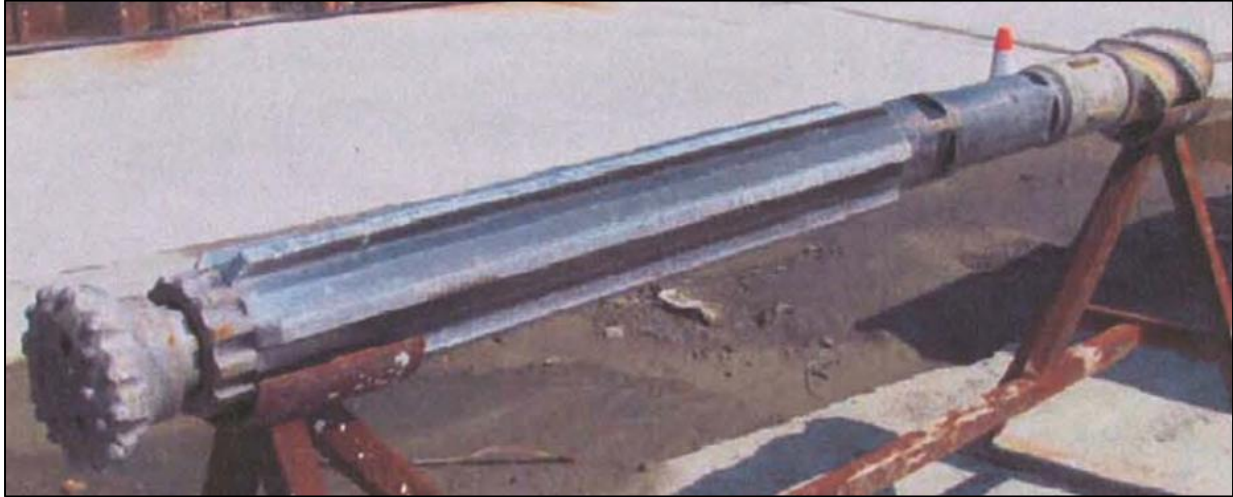
Figure 4-6. Large Water Hammer Down Hole Drill.
