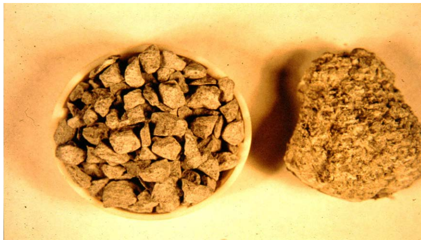
Figure 5-4. Stemming Material Compaction Immediately Above Charge Before (left) and After (right).
