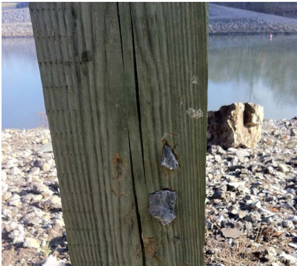
Figure 6-14. Flyrock Embedded in Wooden Post after Boulder Blasting.
