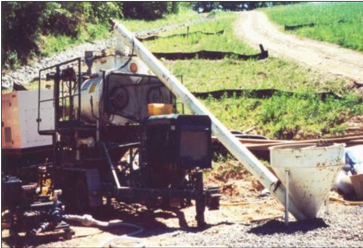
Figure 21-1. Double-drum paddle mixer with a cement auger feed and foaming device (lower left).
