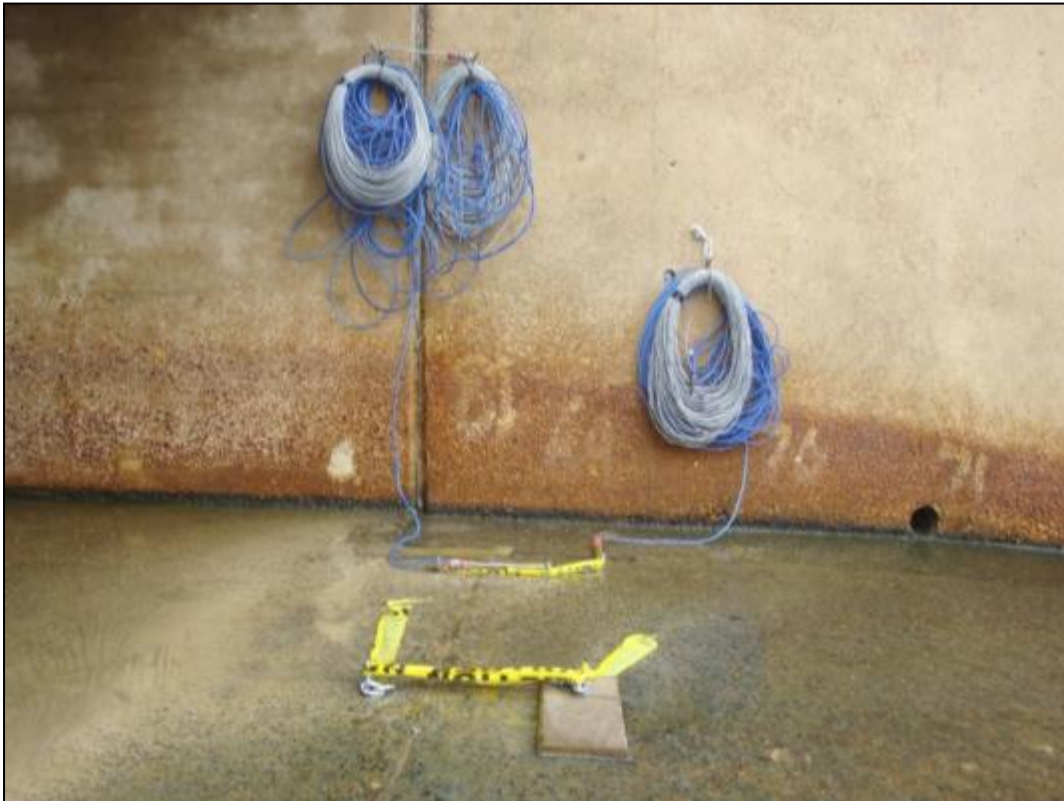
Figure 25-6. Crack displacement devices installed at the spillway wall and parabolic slab at Barker Dam west of Houston, TX (Galveston District). The instruments were monitored in real time during grouting to ensure that there was no movement or displacement of the walls and slab.
