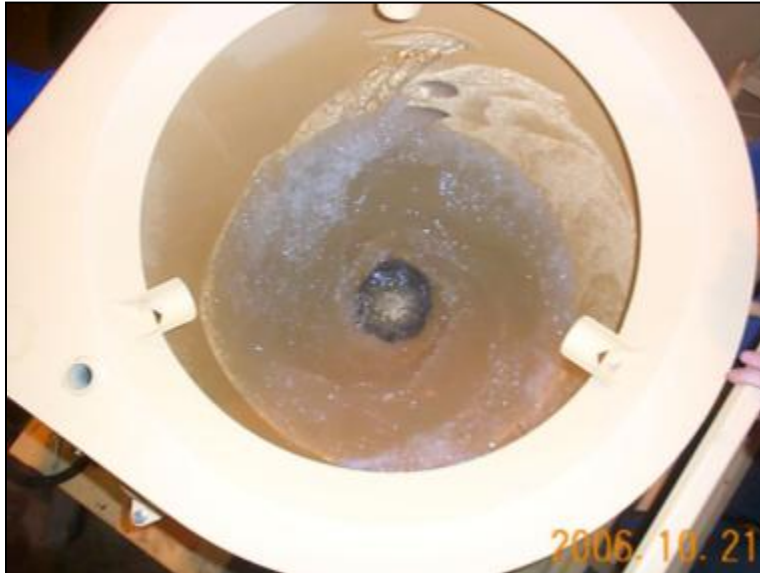
Figure 10-5. Vortex inside a high-shear mixer.
