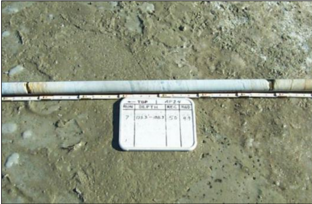
Figure 6-3. Triple-tube core in slightly weathered rock at Mississinewa Dam, IN.
