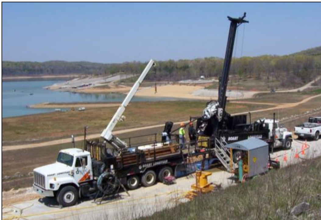
Figure 8-5. Sonic drill with support truck.
