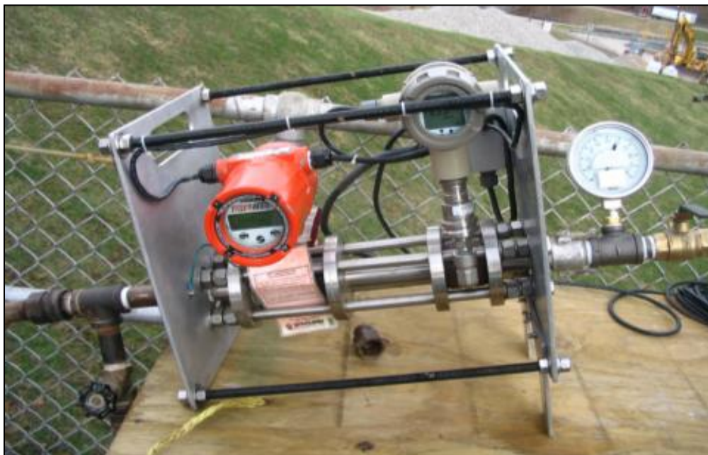
Figure 9-18. Electronic system for flow and pressure readings used in pressure testing.
