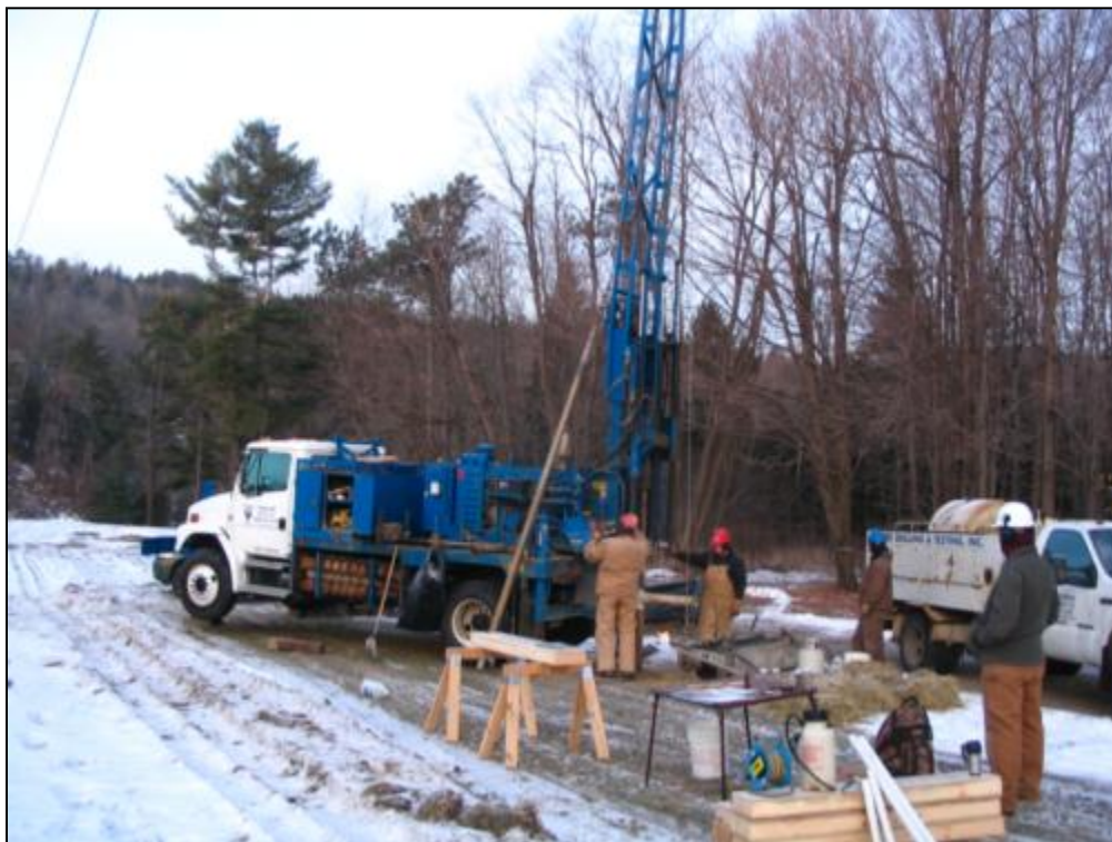
Figure 9-2. Truck-mounted high-speed rotary drill rig.
