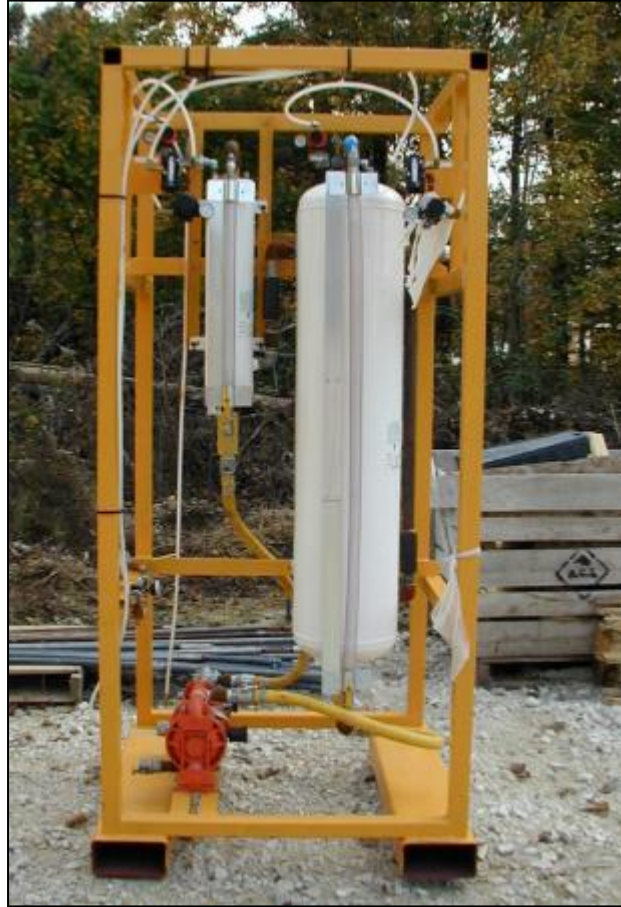
Figure 10-8. Pneumatic additive dispensers.
