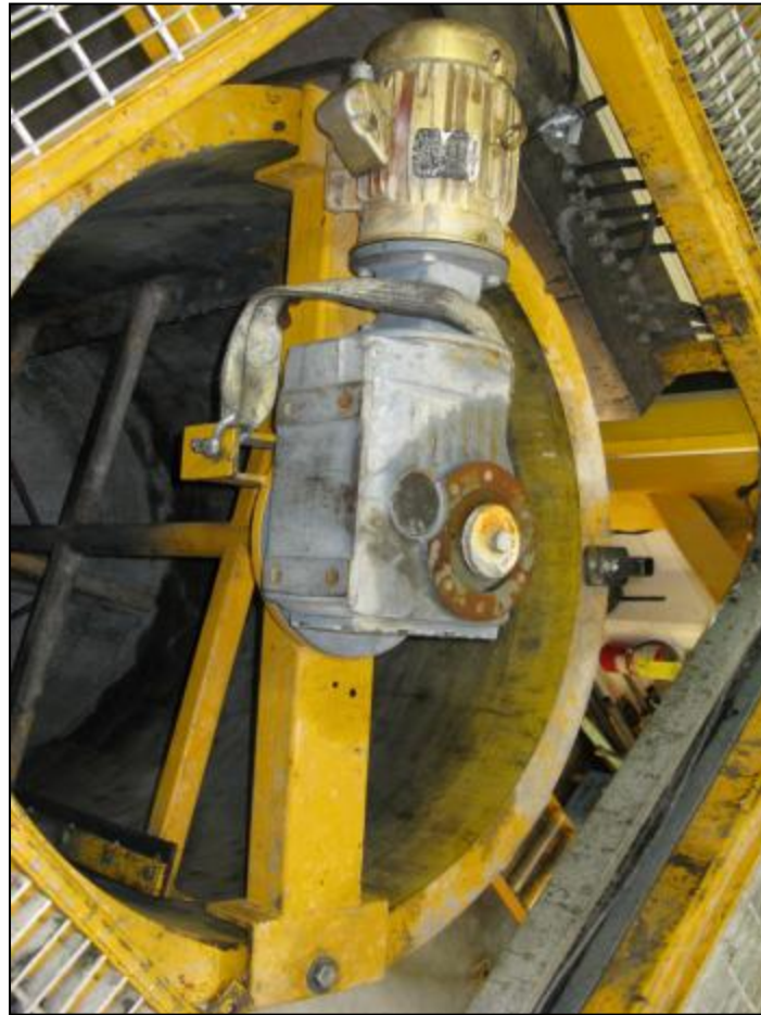
Figure 10-7. Inside view of an agitator tank with a bottom sweeper and other paddles.
