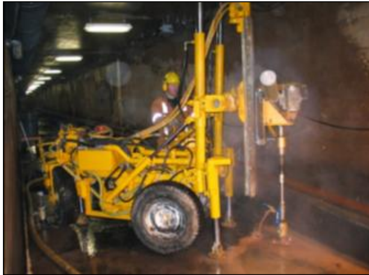
Figure 13-23. Low-clearance pneumatic rotary drill.
