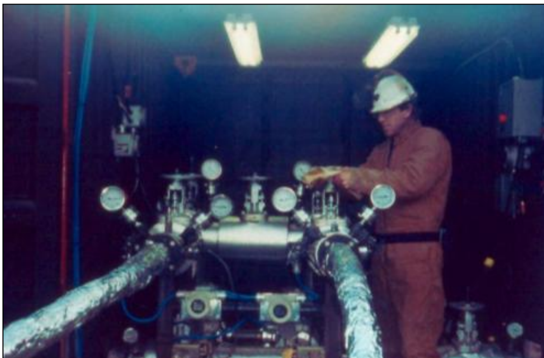
Figure 11-3. Bitumen injection system with insulated piping and instrumentation system.
