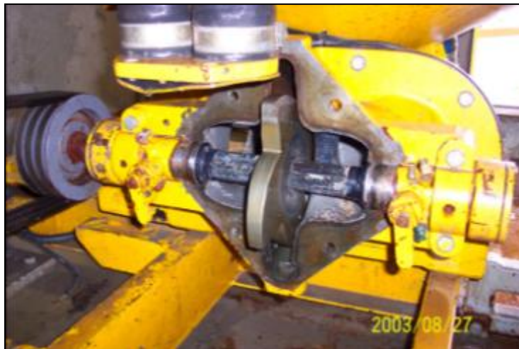
Figure 10-4. Rotor of a high-shear mixer with the mixer cover removed.
