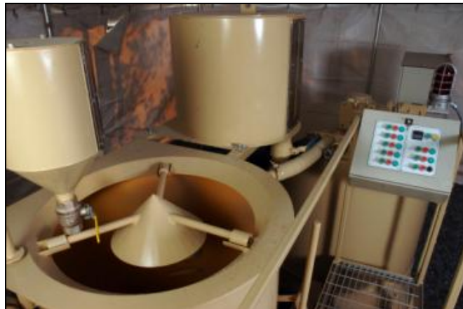
Figure 10-9. Gravity-feed admixture dispenser tanks re-filled via admixture pumps, with a 15-L polymer tank on the left and a 200-L bentonite slurry tank on the right with sight glasses for dosing.
