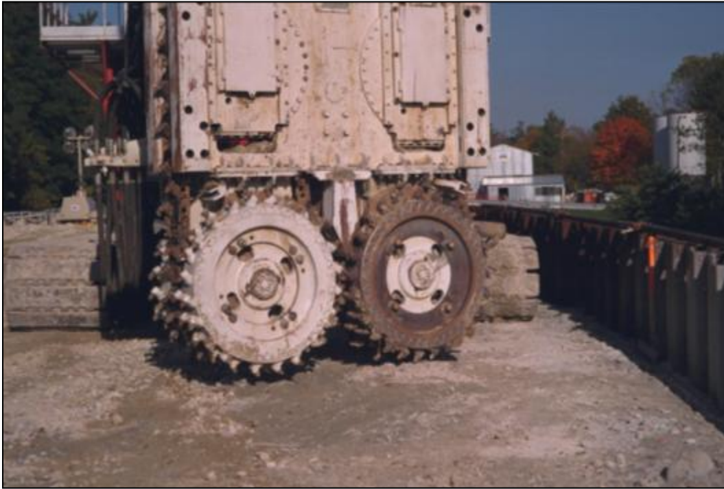
Figure 19-3. Hydromill cutter wheels for limestone excavation at the Mississinewa Dam cutoff wall (Louisville District).
