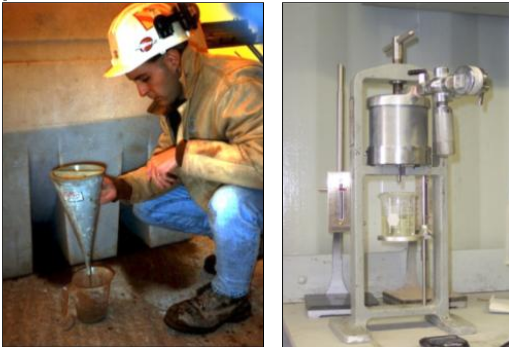
Figure 7-15. Testing for apparent viscosity and pressure filtration.
