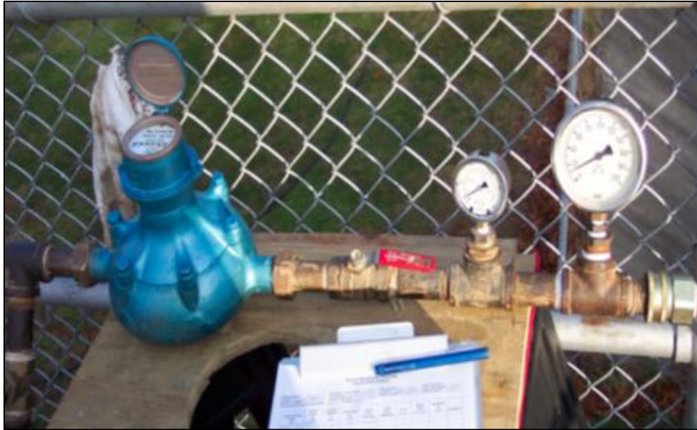
Figure 9-17. Manually read mechanical water meter and pressure gauges for pressure testing.
