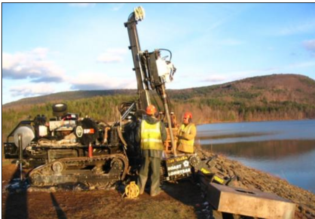
Figure 8-6. Track-mounted sonic rig.
