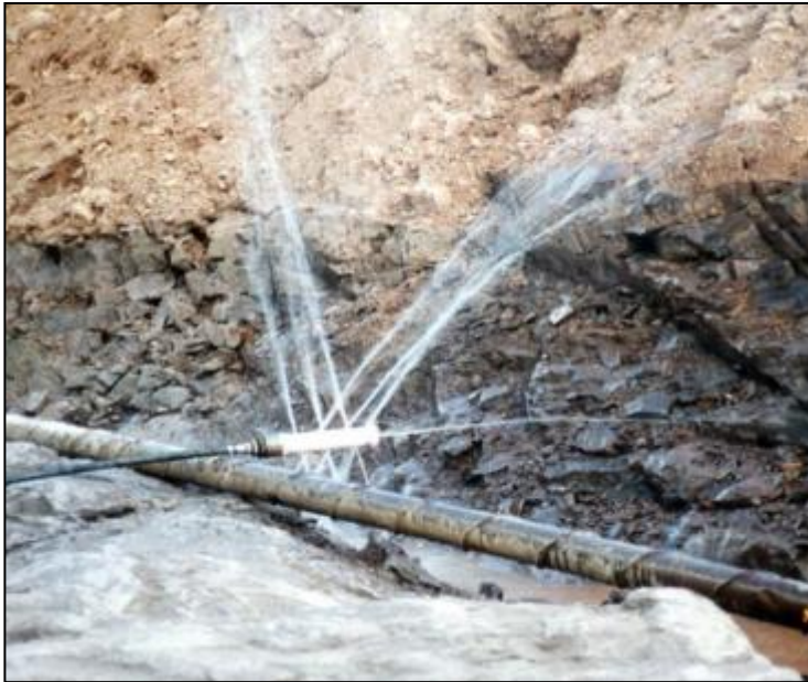
Figure 9-11. Lightweight washout bit and hose for manual applications.
