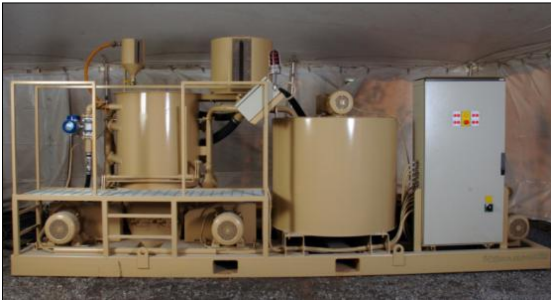
Figure 10-6. 500-L high-shear mixer (on left) with a 1,500-L agitator.
