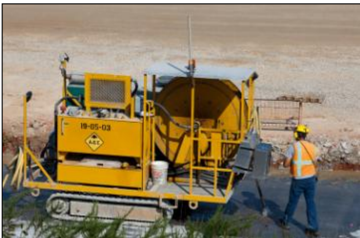
Figure 9-11. Lightweight washout bit and hose for manual applications.
