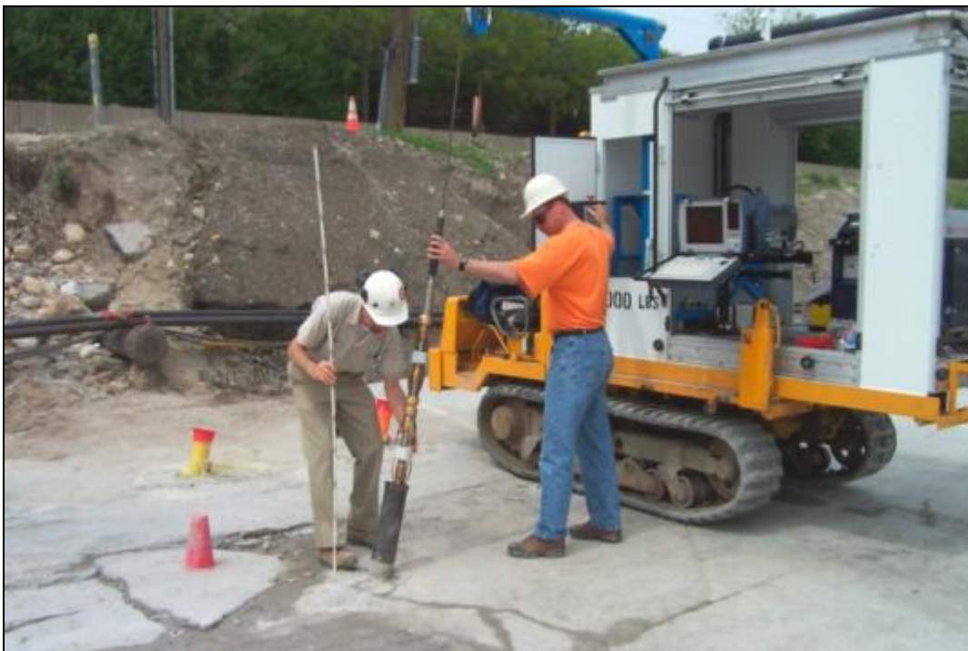
Figure 6-4. Borehole logging system for imaging the borehole sidewall and fractures at McCook Reservoir grouting test section, Chicago, IL.
