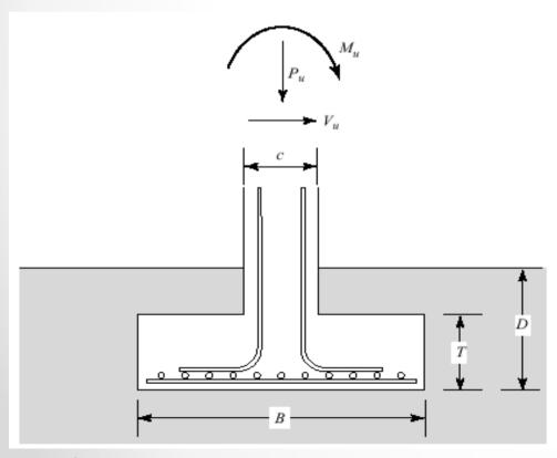
Once geotechnical suitability (stability, bearing capacity, settlement, etc.) is established, the designer must turn to the structural capabilities of the foundation
