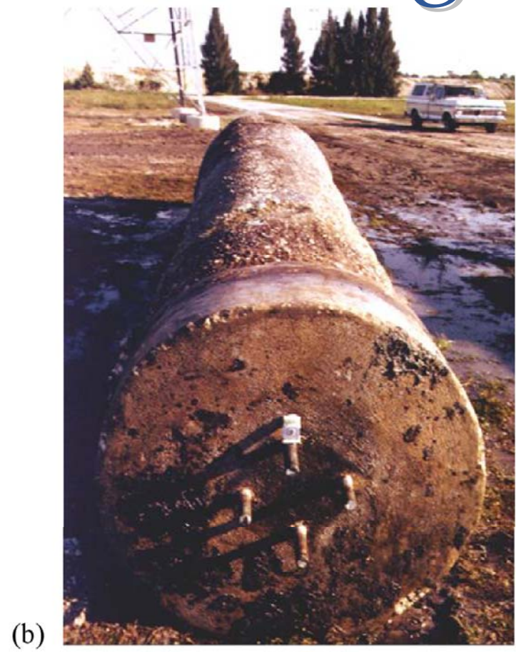
Figure 9-57. Photographs of exhumed shafts (a) shaft where excavation was not adequately cleaned, (b) shaft where excavation was properly cleaned (FHWA, 2002d).
