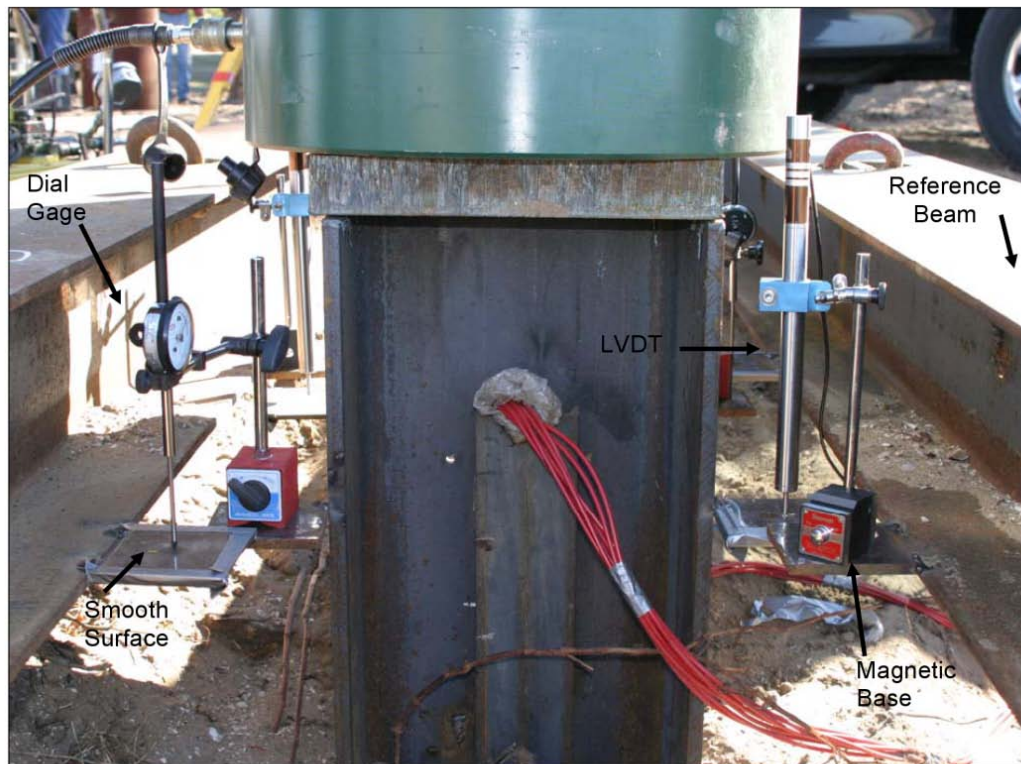
Figure 9-65. Load test movement monitoring components (FHWA, 2006a).
