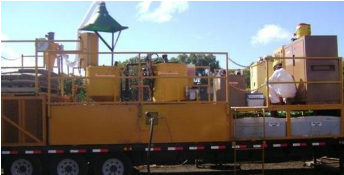
Figure 3.8: Grout plant with two tanks to maintain a continuous supply (courtesy of Applied Foundation Testing).
