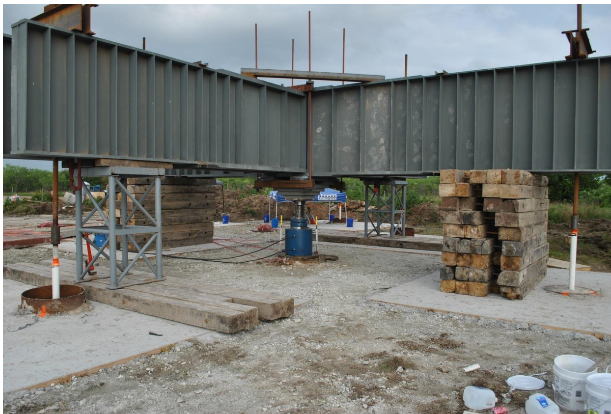
Figure 10.7: Load test setup for top-down loading.
