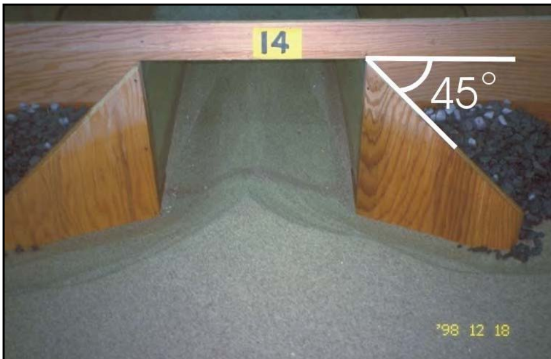
Figure 18.4. Rectangular model with wing walls (Kerenyi et al. 2003).
