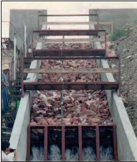
Figure 5.3. Test set up for 1994, d_{50} = 1.27 ft (386 mm).
