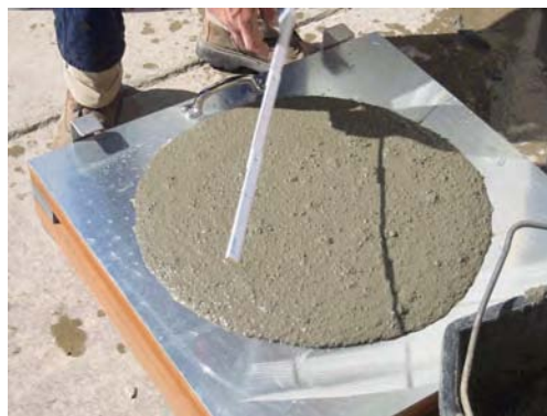
b. Measuring grout slump diameter
