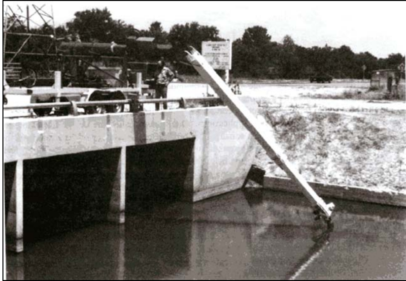
Figure 9.7. FHWA articulated arm in use.
