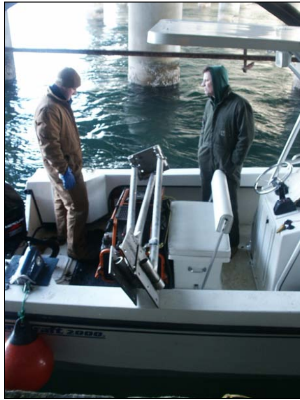
Figure 9.26. Adjustable stainless steel sonar mounting bracket prior to underwater installation.
