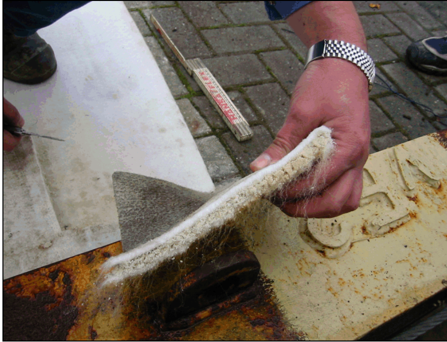
Figure 5.2. Close-up photo of SandMat™ geocomposite blanket. (photo from NCHRP Project 24-07(2), courtesy Colcrete – Von Essen Inc.)
