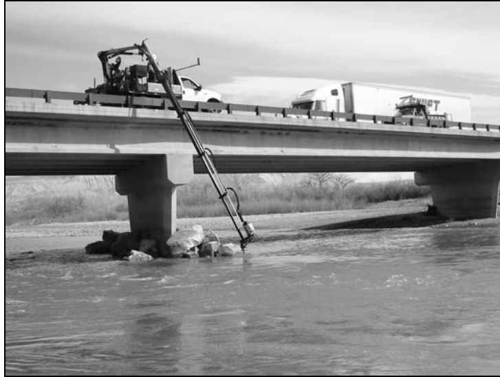
Figure 9.9. Sonar instrument deployed from articulated arm truck.
