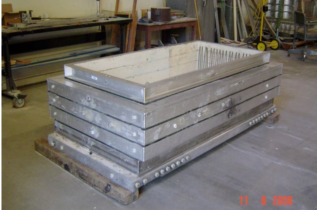
Fig. 2.1 Model container FSB2.
