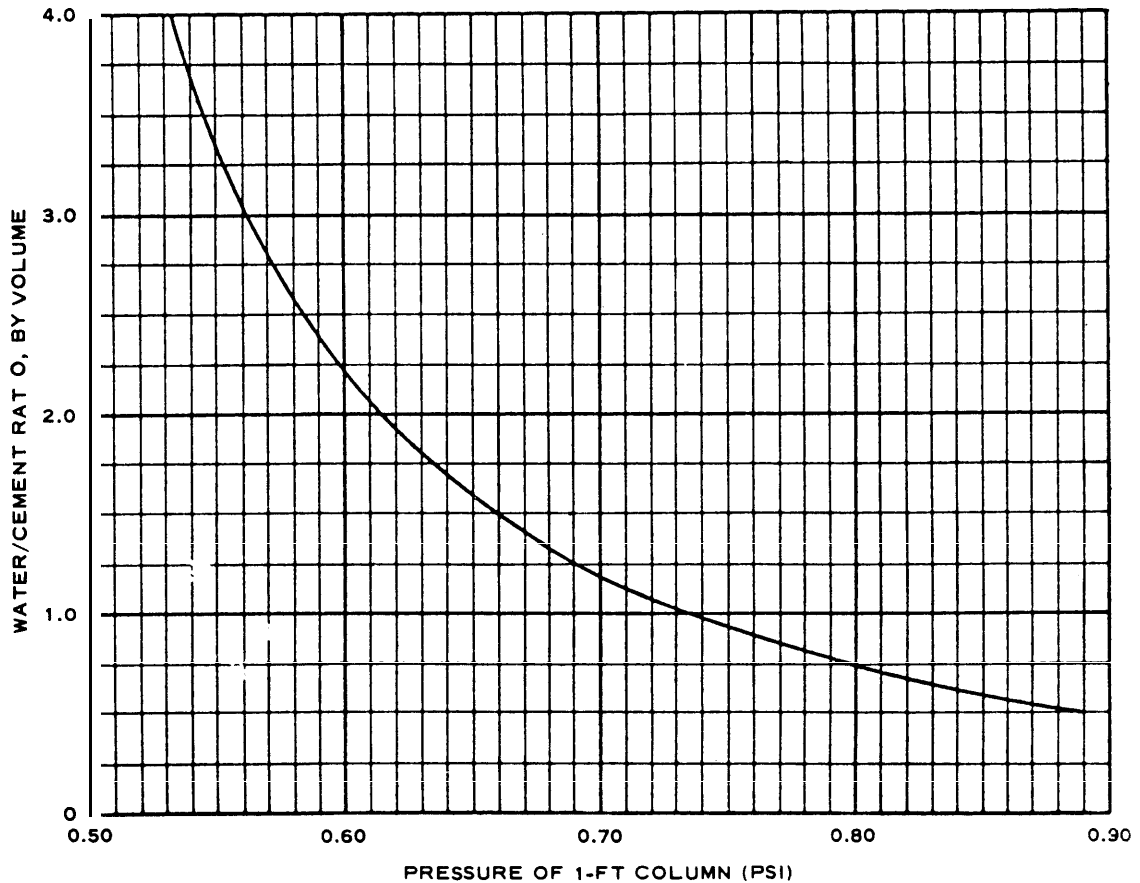
Figure 4. Pressure of neat cement grout
