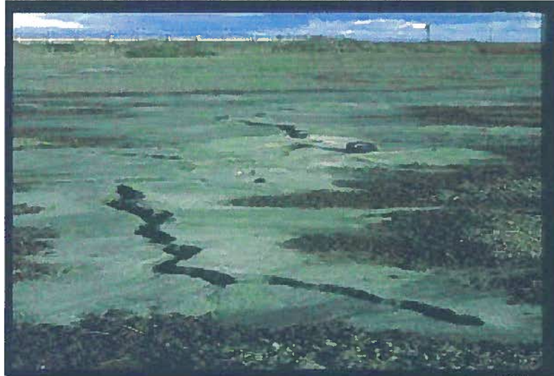
Fig. 8-22: Open crack in liquefied soils in an abandoned channel of the Salinas River, Loma Prieta, California (earthquake: October 17, 1989) (adapted from Yang & Elgamal, 2001).
