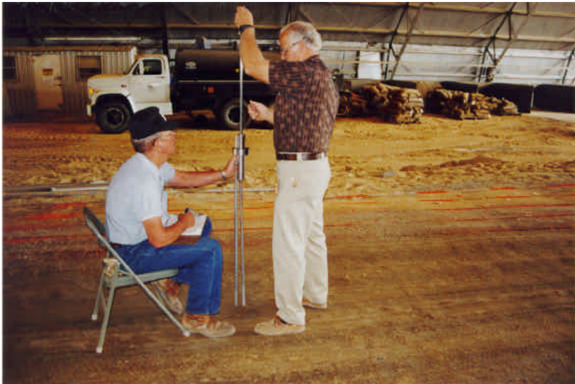
Photo 18. Typical DCP measurements on experiment sections
