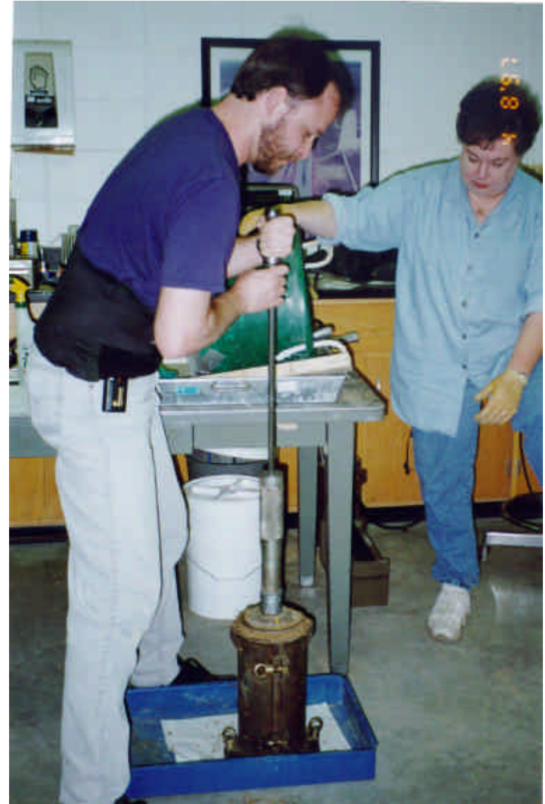
Photo 2. Compacting laboratory test specimens
