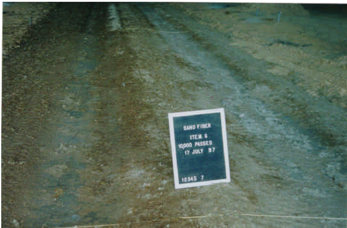
Photo 24. Item 6 of experiment section one after 10,000 truck passes
