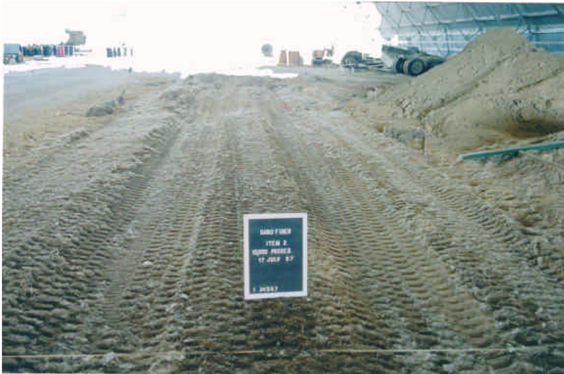
Photo 20. Item 2 of experiment section one after 10,000 truck passes
