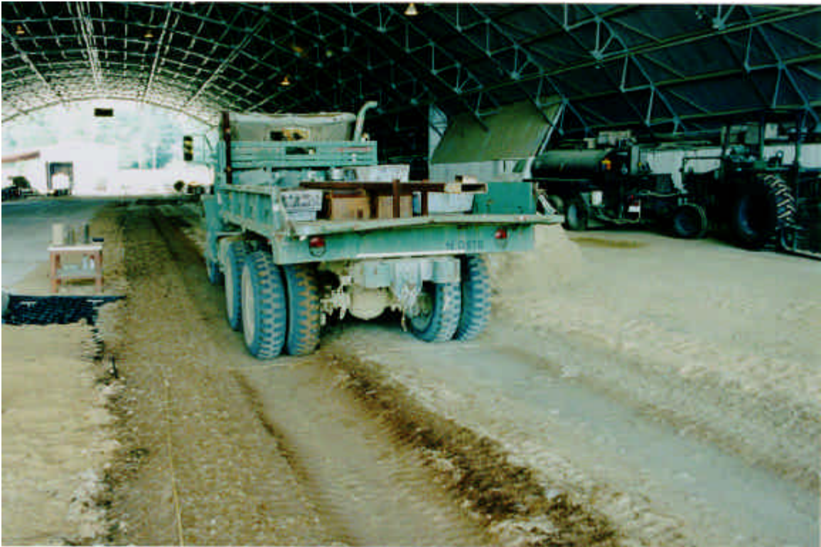
Photo 16. M923 5-ton military truck trafficking experiment section one
