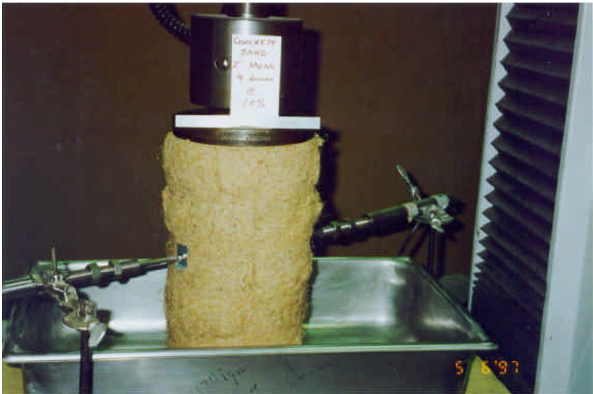
Photo 6. Test on 2-in. Monofilament (4 denier) fibers at 1.0 % fiber content in concrete sand
