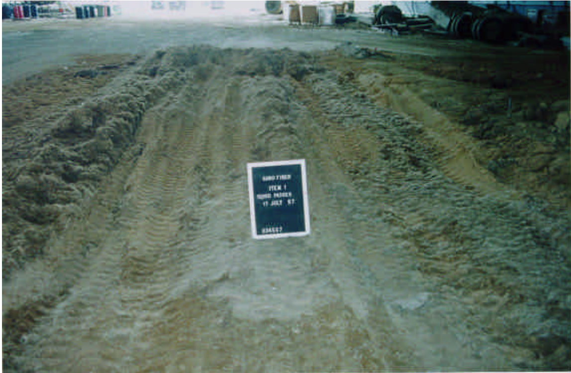
Photo 19. Item 1 of experiment section one after 10,000 truck passes
