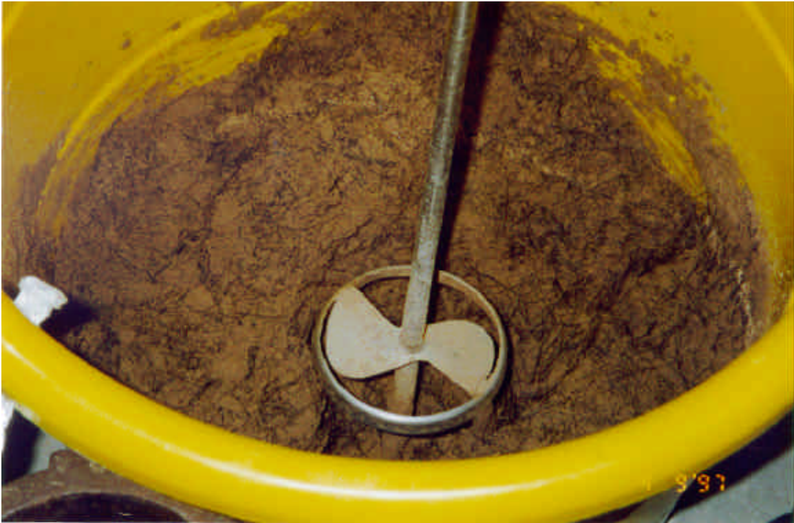
Photo 3. Fibers mixed in concrete sand in the laboratory
