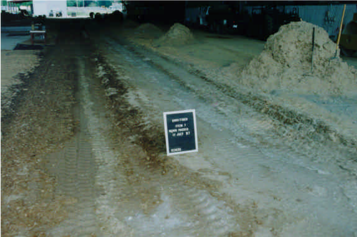
Photo 25. Item 7 of experiment section one after 10,000 truck passes
