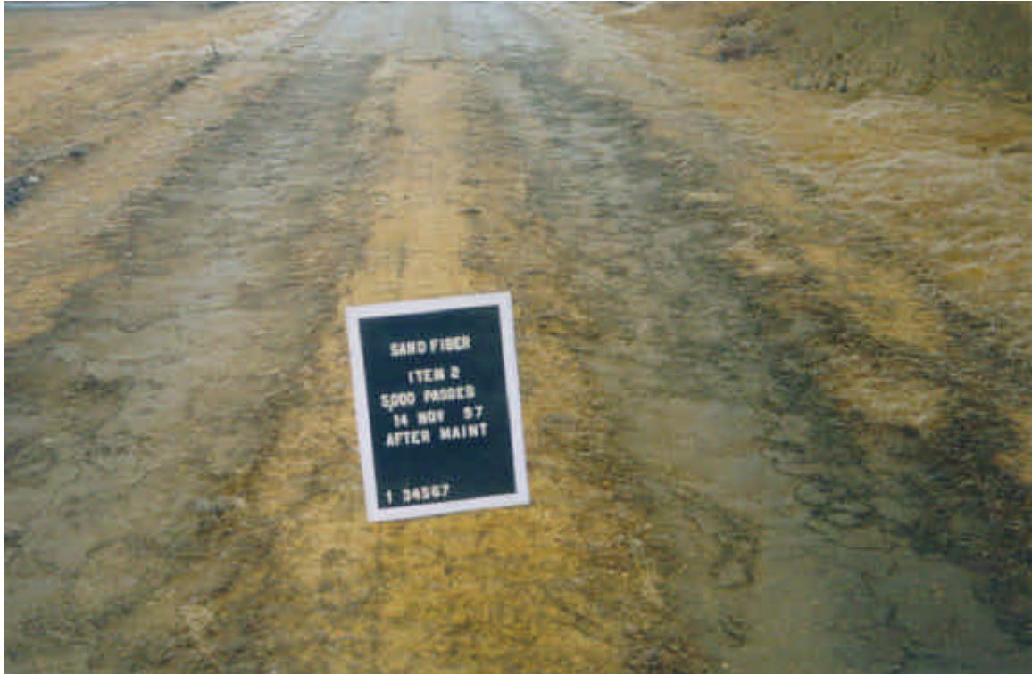
Photo 27. Item 2 of section two — 5,000 truck passes after maintenance
