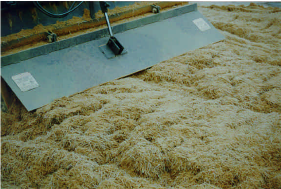
Photo 10. Uniform mixture of tape fibers in concrete sand
