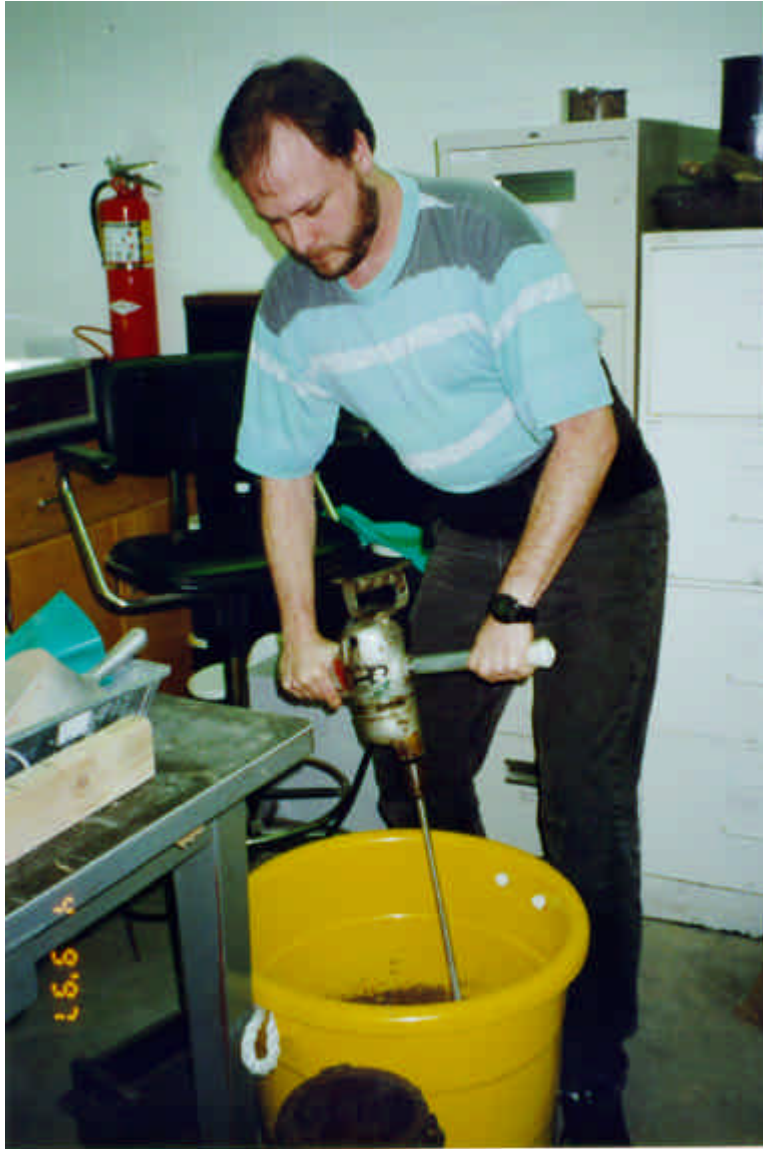
Photo 1. Mixing fibers into the sand in the laboratory
