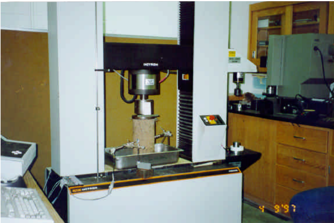
Photo 4. Laboratory unconfined compression test setup
