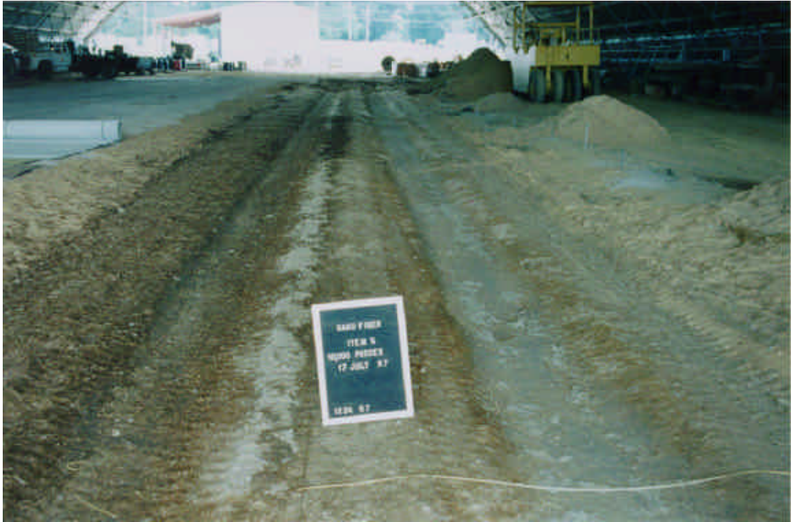
Photo 23. Item 5 of experiment section one after 10,000 truck passes
