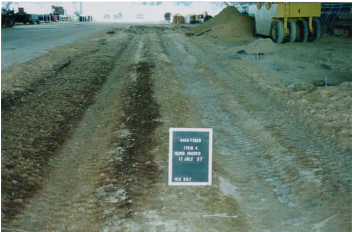
Photo 22. Item 4 of experiment section one after 10,000 truck passes
