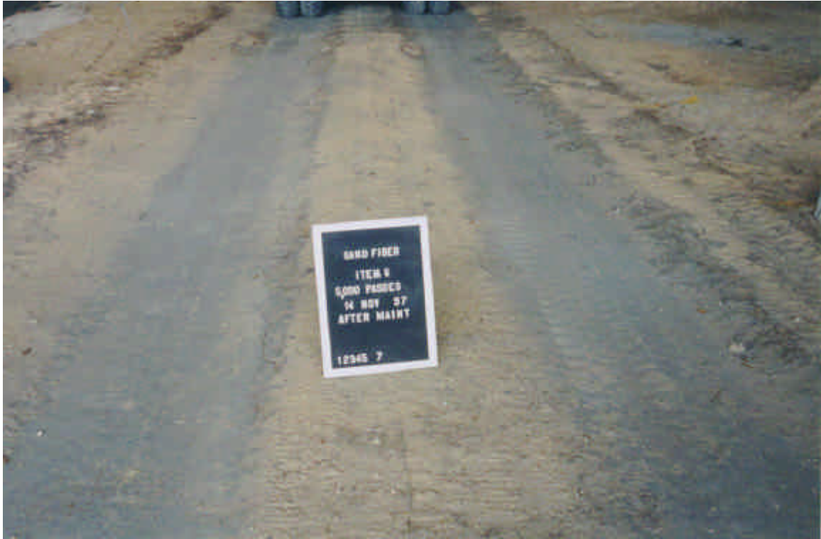
Photo 31. Item 6 of section two — 5,000 truck passes after maintenance
