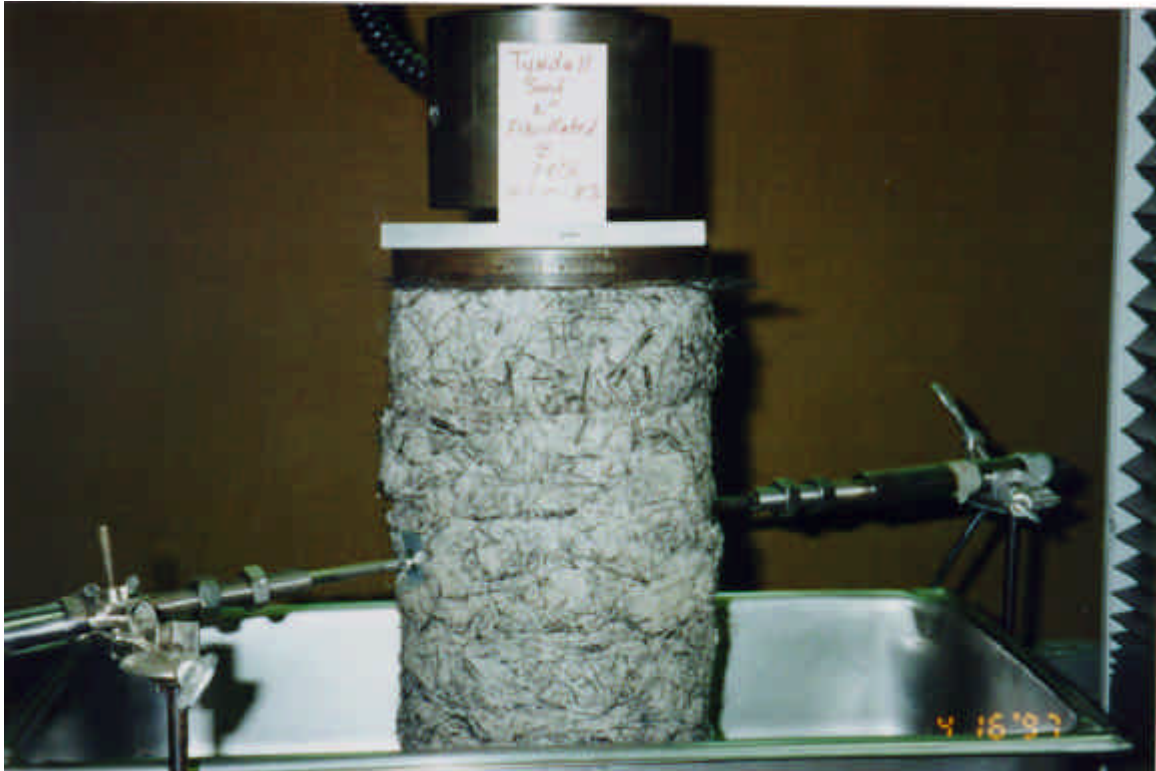
Photo 7. 2-in. Fibrillated fibers at 1.0 % fiber content in Tyndall AFB sand during testing
