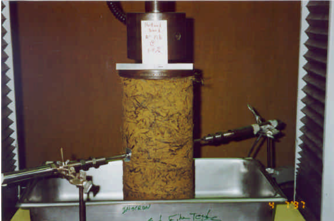
Photo 5. 2-in. Fibrillated fibers at 1.0 % fiber content in Holland LZ silty sand prior to testing
