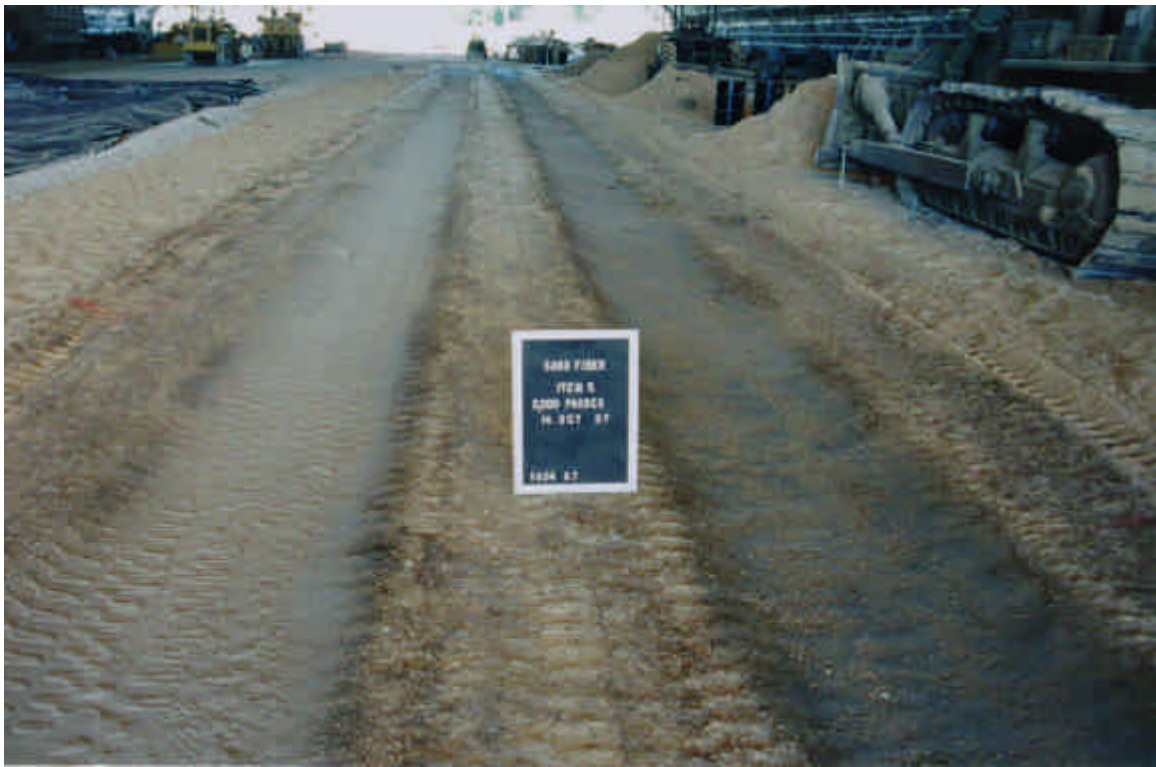
Photo 30. Item 5 of section two — 5,000 passes before maintenance
