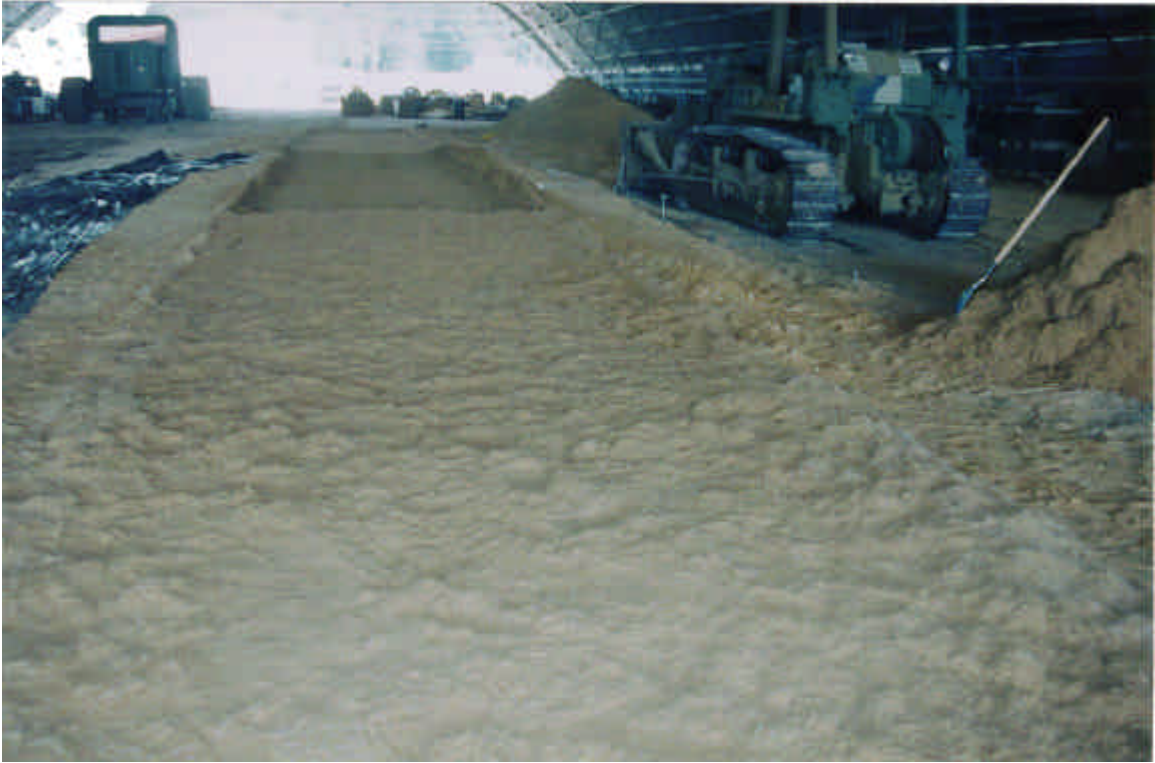
Photo 11. Leveled experiment item prior to compaction
