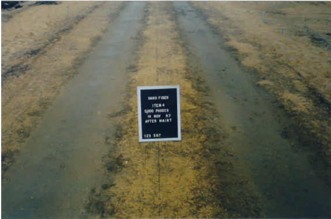
Photo 29. Item 4 of section two — 5,000 truck passes after maintenance
