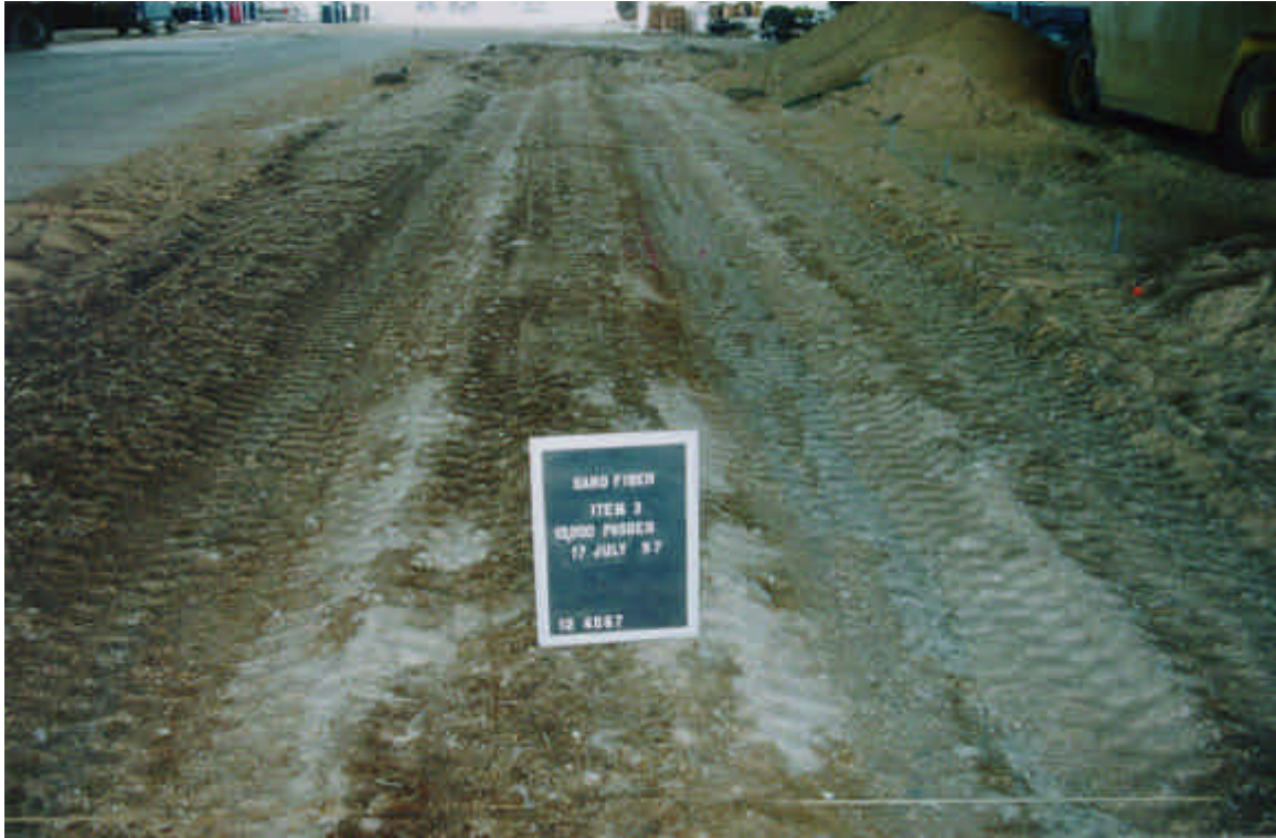
Photo 21. Item 3 of experiment section one after 10,000 truck passes
