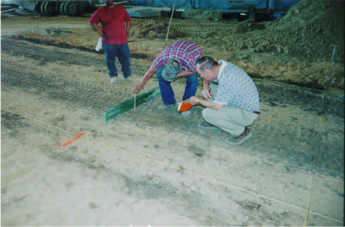
Photo 17. Rut depth measurements on item 1 of experiment section one
