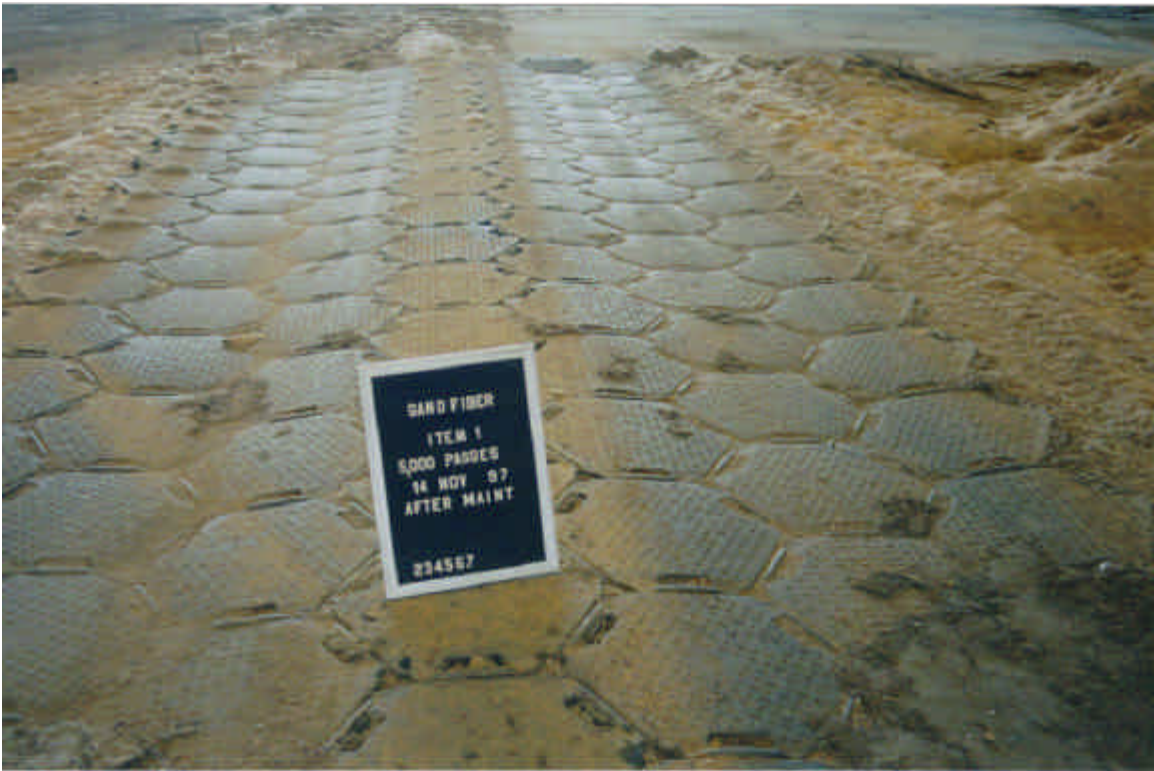
Photo 26. Item 1 of experiment section two — 5,000 passes after maintenance
