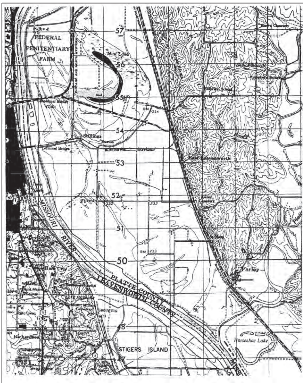
Figure 3-9. Channel bar deposits, oxbow lakes, and backswamp/floodplain deposits
