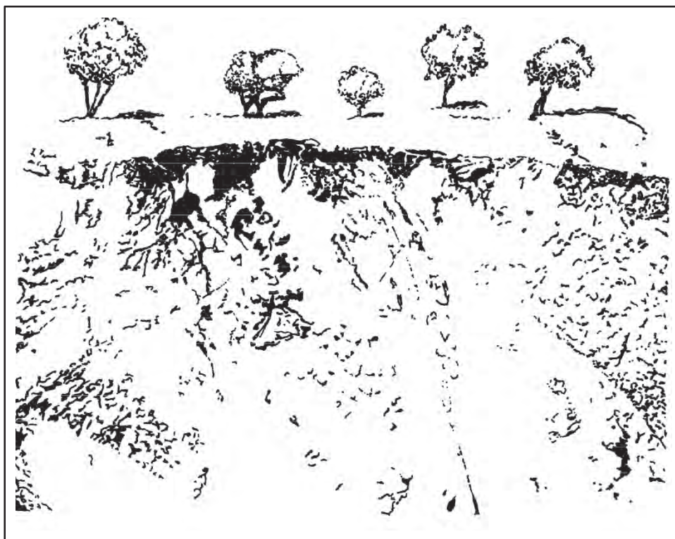
Figure 4-1. Residual soil forming from the in-place weathering of igneous rock
