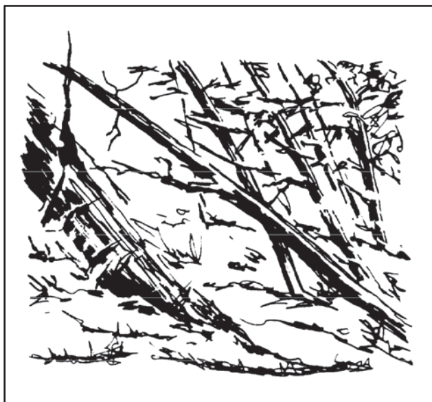
Figure 10-8. Backward rotation of a slump block
