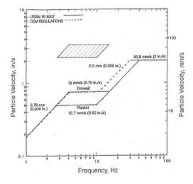
Figure 1. Safe level blasting criteria from USBM RI 8507 and the derivative version (dashed line), the Chart Option from OSM surface coal mine regulations. Shaded area shows maximum velocities of structural vibrations with amplification of 4.5 at resonance. Data were modified from Siskind (2000) and plot was adapted from Svinkin (2008). Reprinted with permission.
