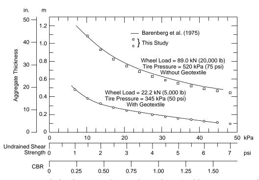
Figure 11. Static loading design curves from Barenberg et al. (1975) and design points generated for this report according to method documented in Appendix B.
