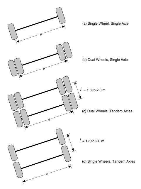
Figure 4. Wheel and axle configurations.
