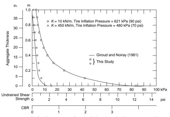
Figure 13. Static loading design curves with geotextiles from Giroud and Noiray (1981) and points generated for this report according to method documented in Appendix B.
