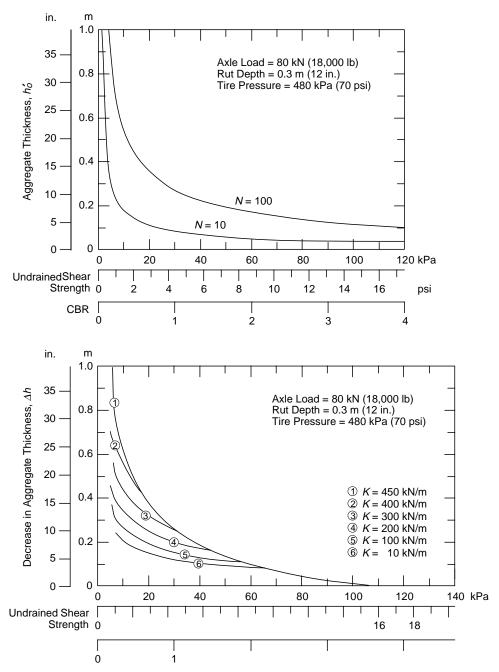
Figure 6. Aggregate thickness,  $h_0'$  (top), and reduction of aggregate thickness,  $\Delta h$  (bottom), resulting from use of geotextile as a function of soil cohesion for 12-in. rut depth. N is number of vehicle passes and K is tensile modulus of geotextile. (From Giroud and Noiray 1981.)
