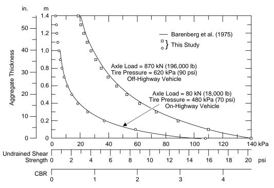
Figure 12. Static loading design curves without geotextile from Giroud and Noiray (1981) and points generated for this report according to method documented in Appendix B.
