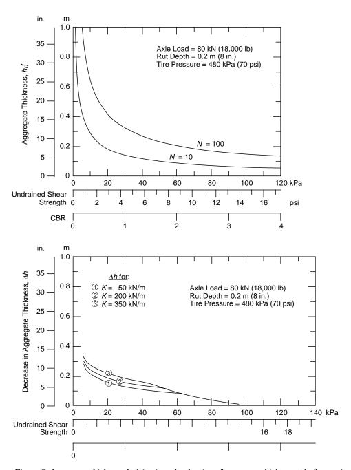
Figure 7. Aggregate thickness,  $h_o{'}$  (top), and reduction of aggregate thickness,  $\Delta h$  (bottom), resulting from use of geotextile as a function of soil cohesion for 8-in. rut depth. N is number of vehicle passes and K is tensile modulus of geotextile. (From Holtz and Sivakugan 1987.)
