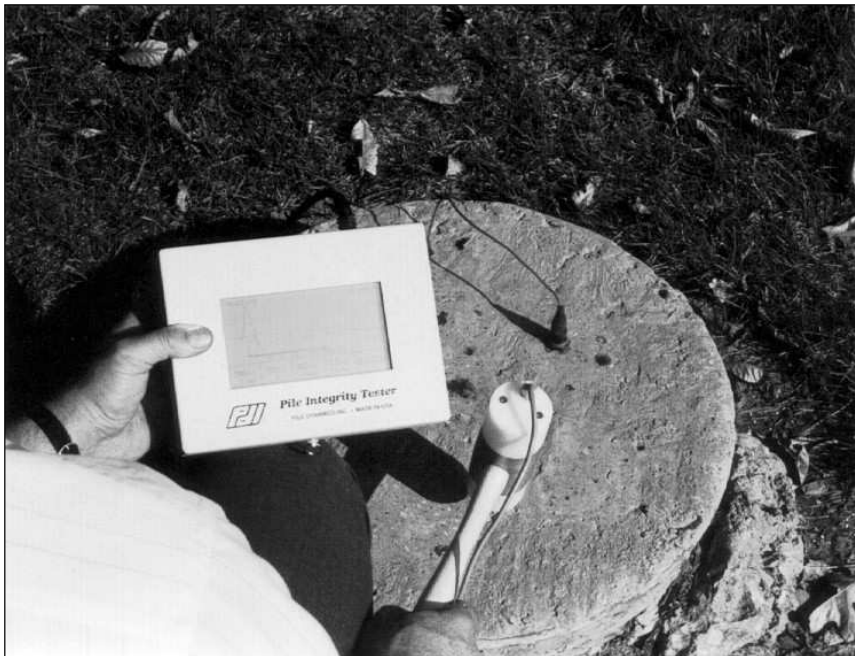
Figure 39, Pile Integrity Tester (After PDI, 1993)
