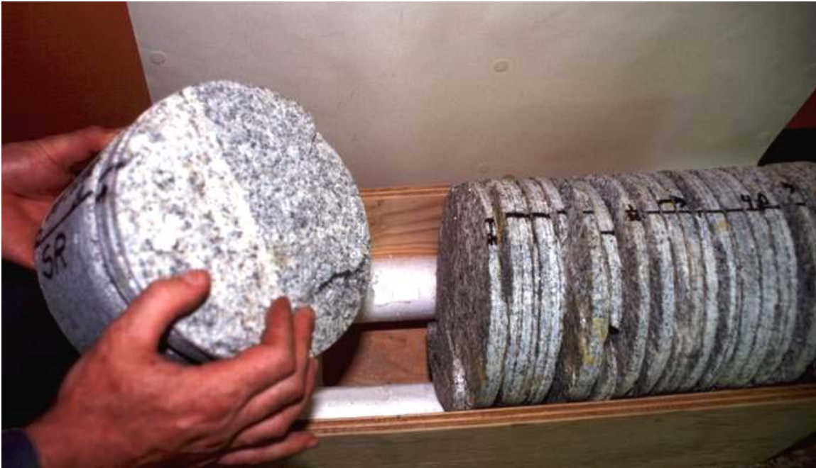
Figure 1.7: Diking of a 150 mm core of granite as a result of high in situ stresses.
