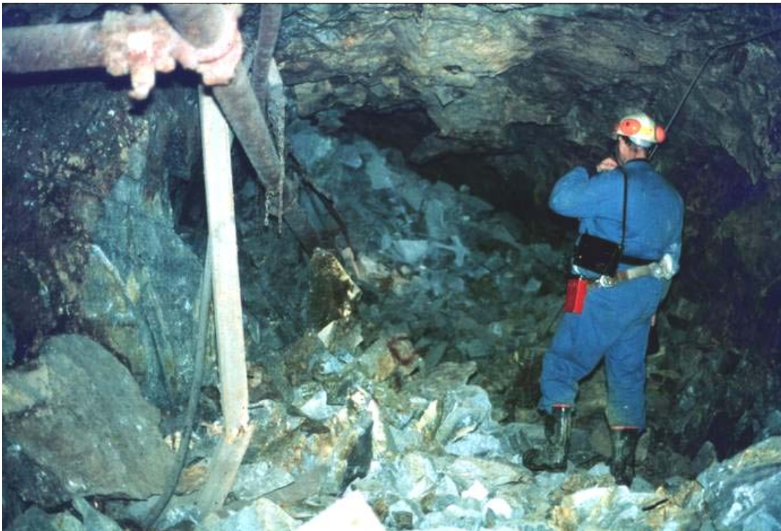
Figure 1.2: The results of a rockburst in an underground mine in brittle rock subjected to very high stresses.
