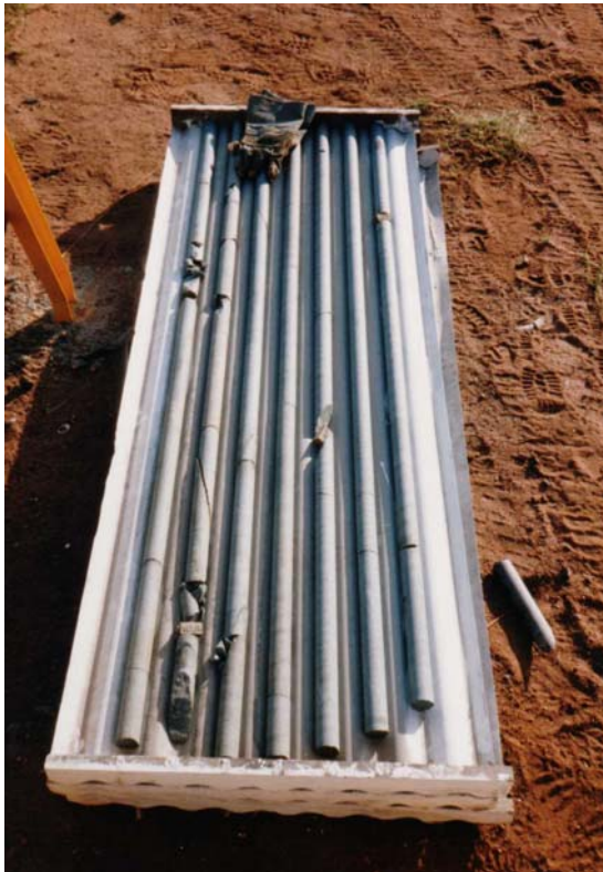
Figure 11.20: Excellent quality core with very few discontinuities from the massive gneiss of the Rio Grande project in Argentina.
