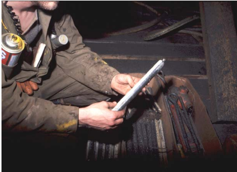
Figure 14.3: Typical two-component resin cartridge used for anchoring and grouting rockbolts.
