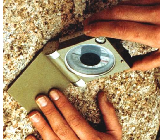
Cocla – Geological Stratum compass
