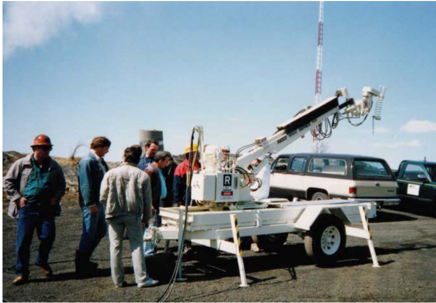
Figure 15.10: Compact trailer-mounted robot unit for remote controlled shotcrete application.
