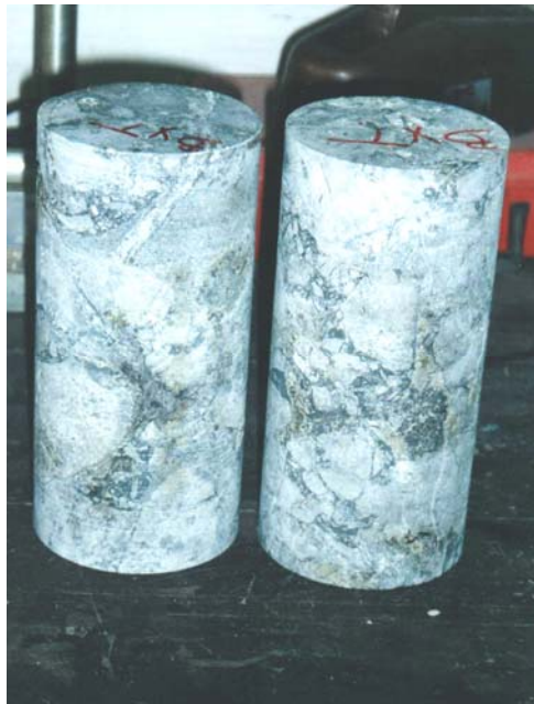
Fig. 11.19. 100 mm diameter by 200 mm long specimens of Braden Breccia from the El Teniente mine in Chile.
