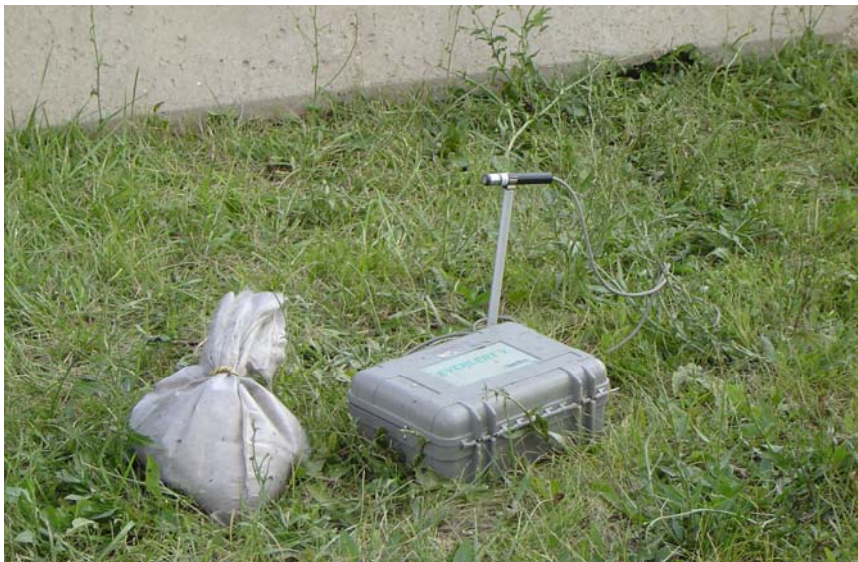
Figure 16. Vibra-tech Everlert VE monitoring device and ballast at Static Load Test Site F
