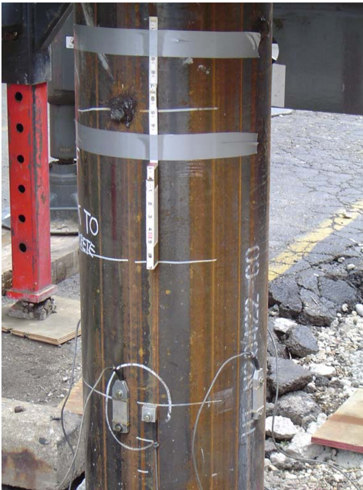
Figure 11. HSDPT transducers on a pile to be tested during restrike.
