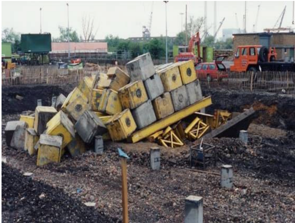
Figure 2.2 Platform bearing failure under kentledge test
