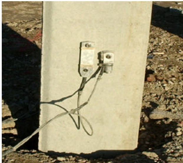
Figure 5.9 Strain gauge and accelerometer bolted to precast concrete pile The arrangement is repeated on the opposite pile shaft face
