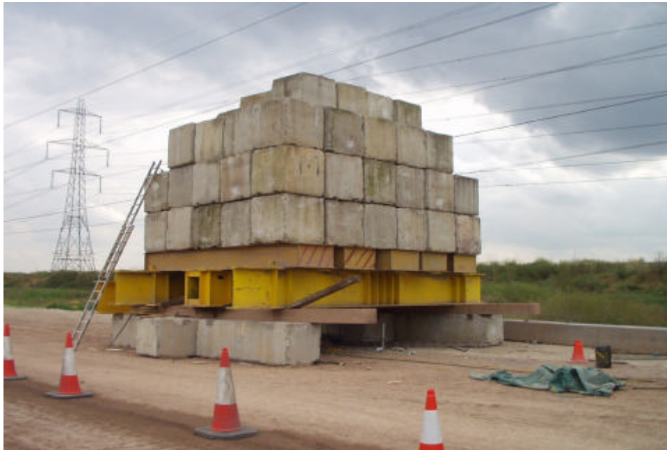
Figure 5.3 3MN kentledge test
