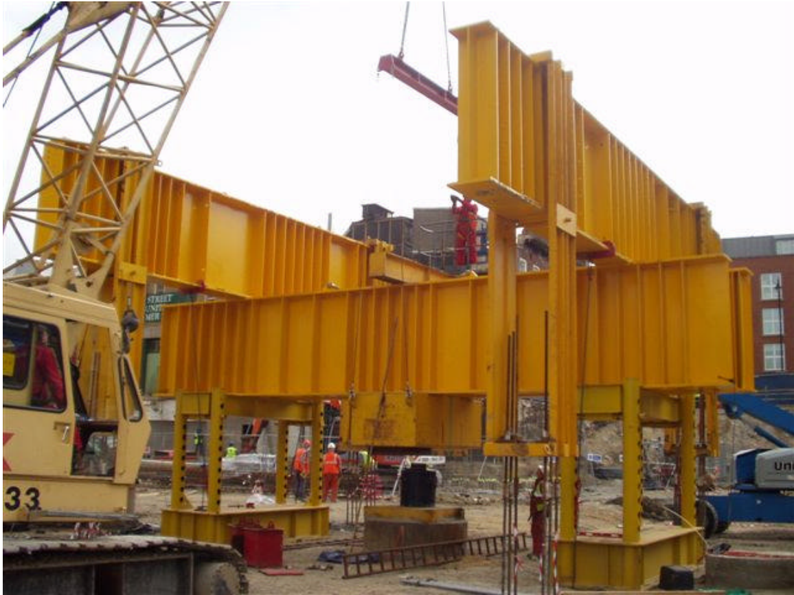
Figure 5.1 30MN reaction pile test
