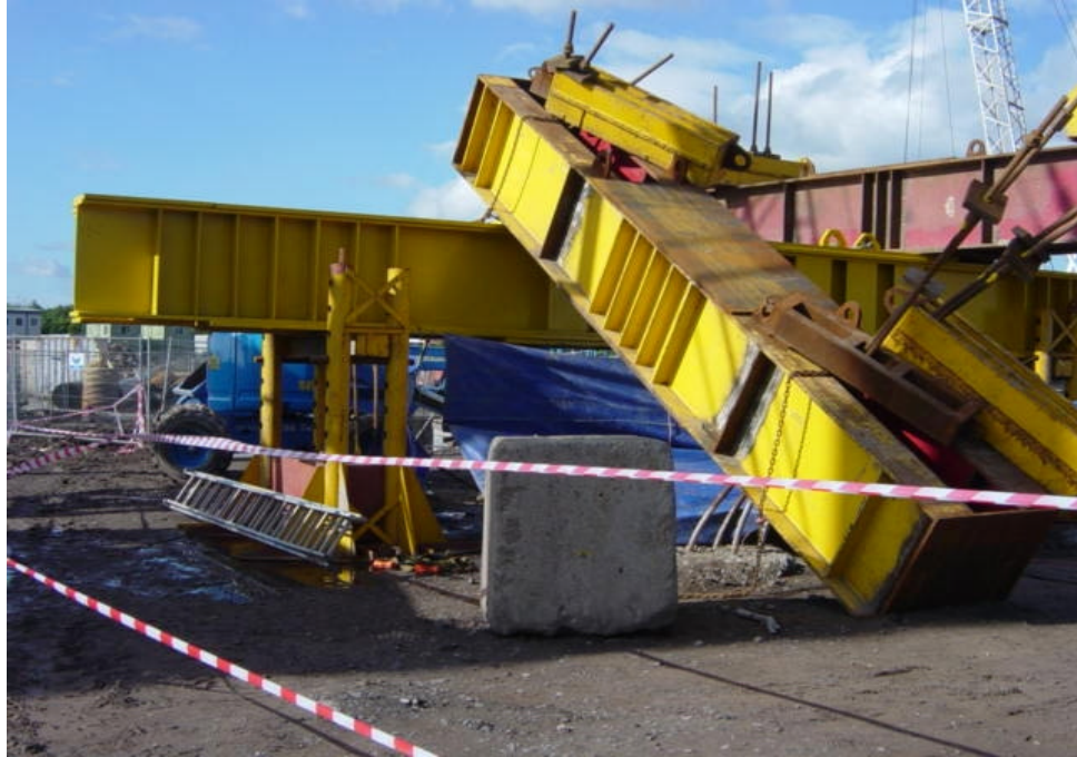
Figure 2.1 Failure of tension bar system in reaction pile
