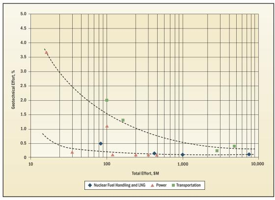
Figure 3. Geotechnical Cost as a Function of Total Project Estimated Cost
