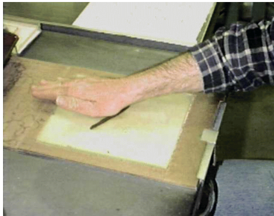
Figure 2: Rolling the plastic limit sample on the rolling surface.
