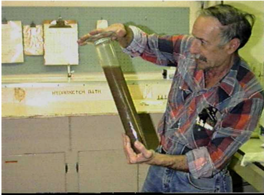
Figure 3: Agitating slurry in the sedimentation cylinder.
