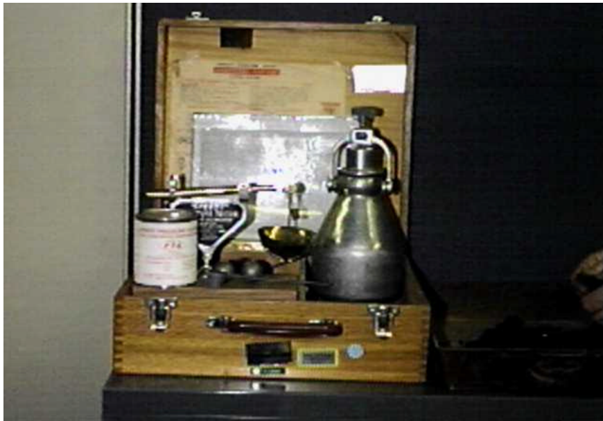
Figure 1. Calcium carbide moisture testing kit with associated equipment.
