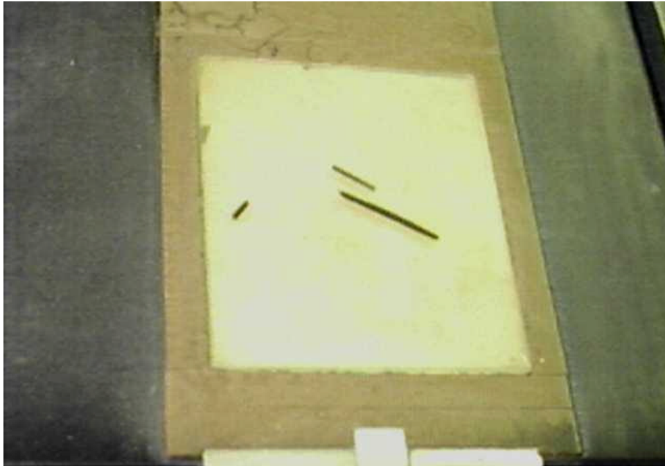
Figure 3: Roll into 3.2 mm diameter thread.
