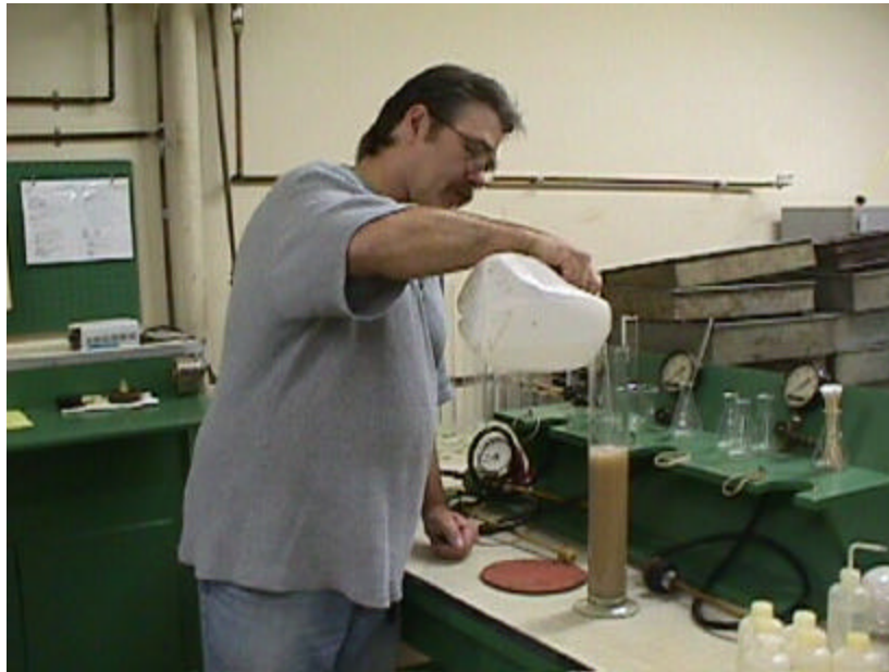
Figure 2: Adding water to the calibration mark on the cylinder.
