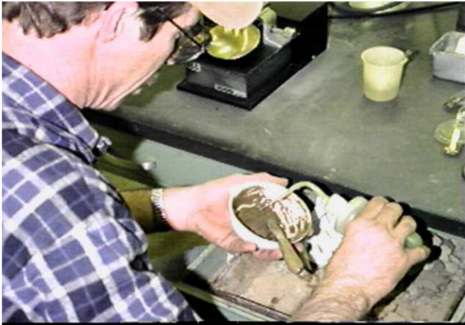
Figure 4: Add small increments of water when sample nears liquid limit.
