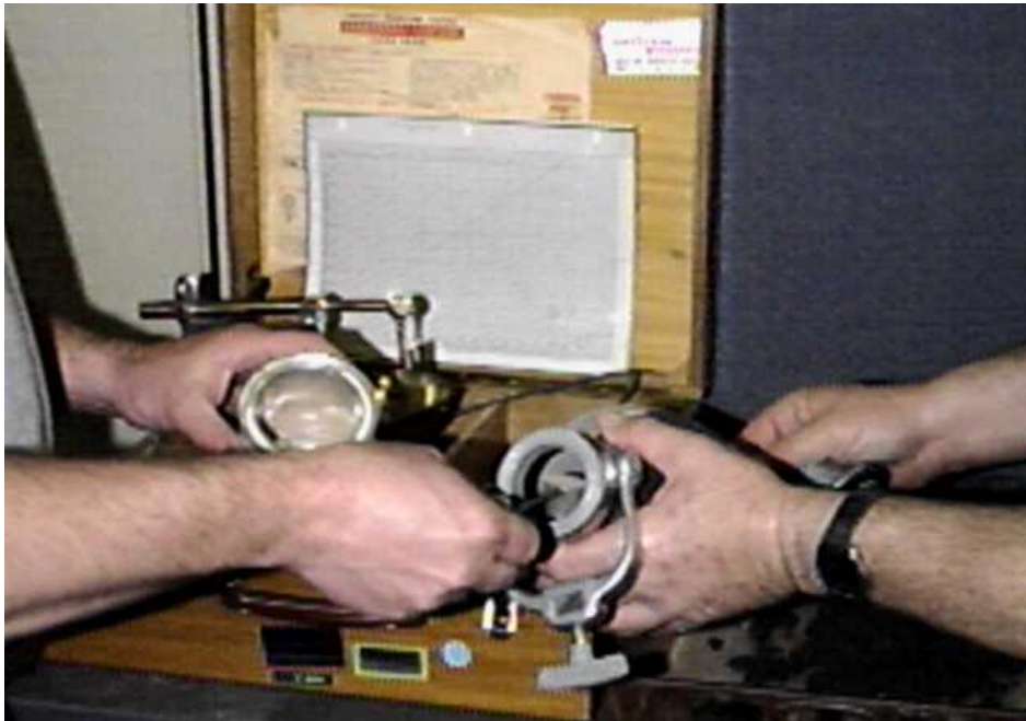
Figure 2. Placing calcium carbide into moisture tester chamber.
