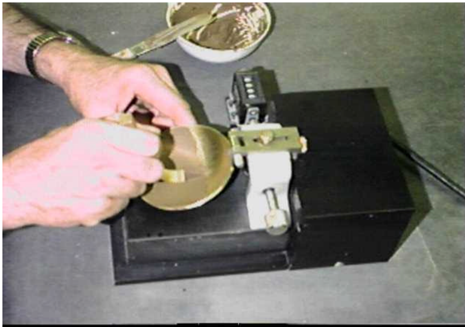
Figure 6: Dividing soil with AASHTO grooving tool.
