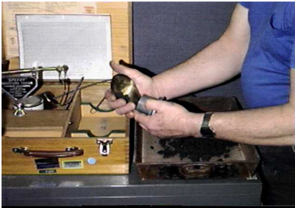
Figure 3. Placing moist soil sample inside the cap of meter.
