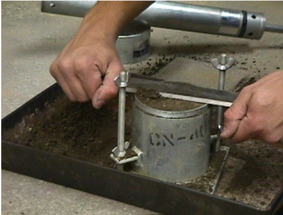
Figure 5: Sawing motion removes material above the top of the mold.
