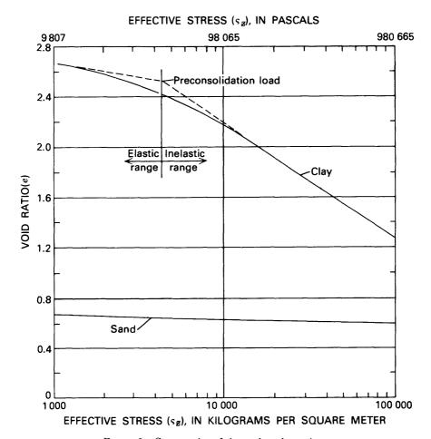
FIGURE 3.—Compression of clay and samples.
