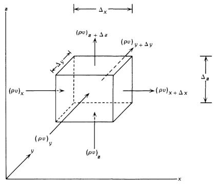
FIGURE 1.-Elemental volume of a saturated porous medium.
