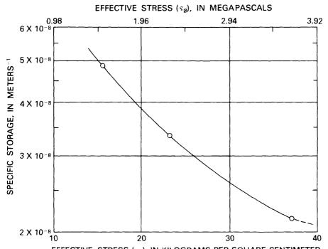
EFFECTIVE STRESS ( $s_{\vec{x}}$ ), IN KILOGRAMS PER SQUARE CENTIMETER FIGURE 6.—Specific storage and effective stress.
