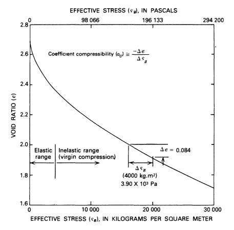
FIGURE 4.-Compression of a clay sample.
