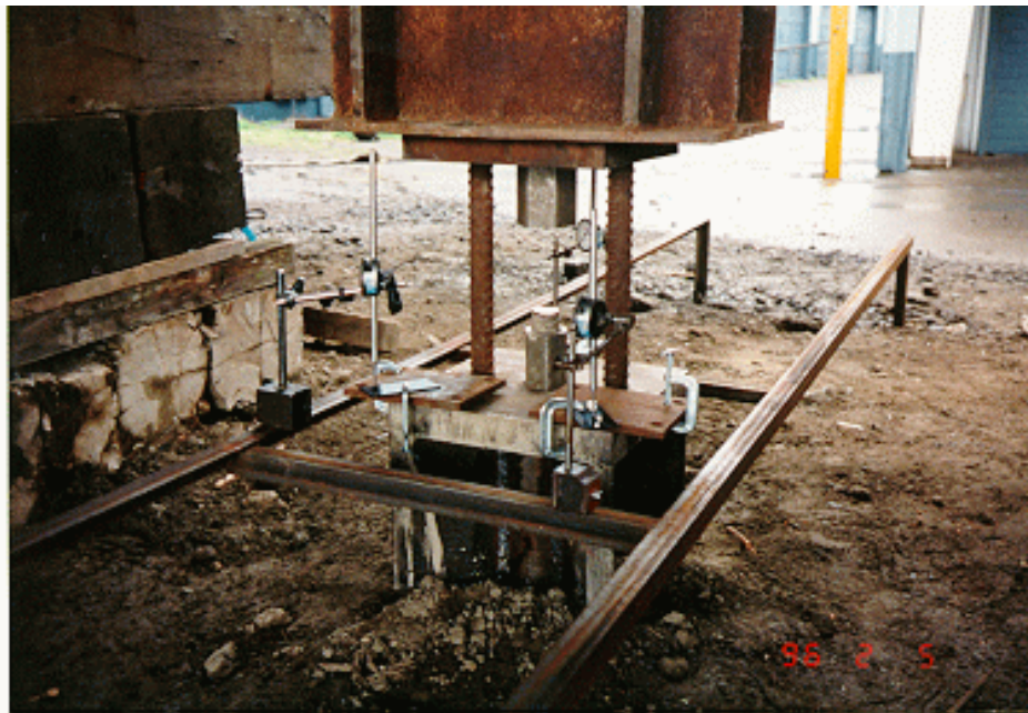
Photograph 7 - 6. Micropile Load Test Instrumentation
