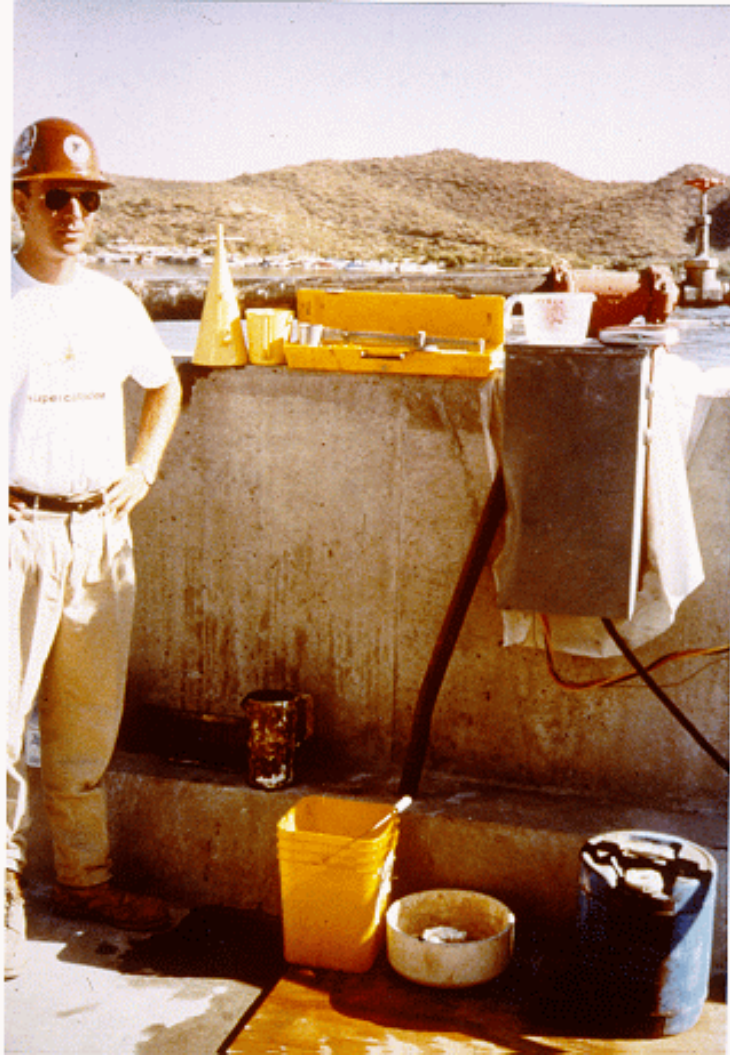
Photograph 8 - 7. Baroid Mud Balance Test
