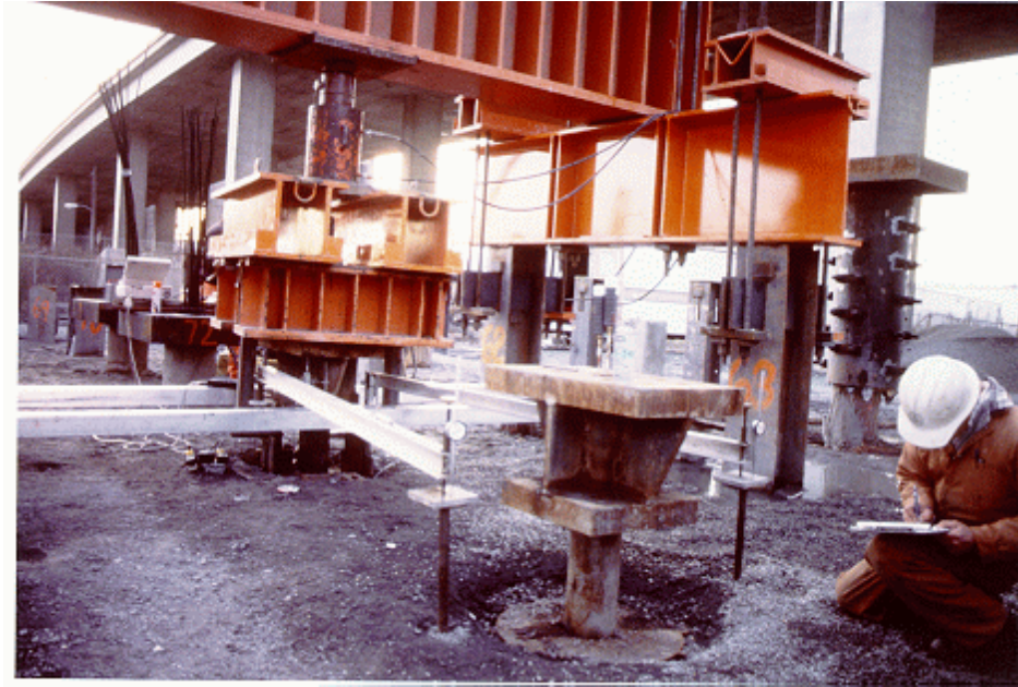
Photograph 7 - 5. Micropile Load Test Instrumentation
