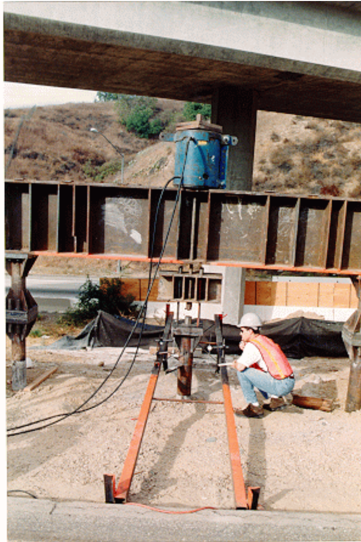
Photograph 7 - 2. Tension Load Test Setup
