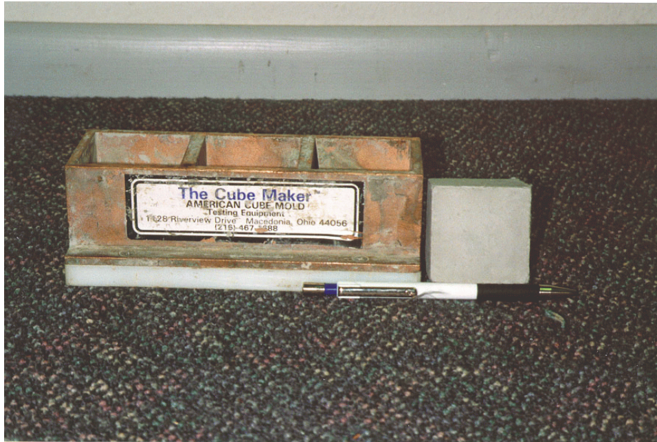
Photograph 8 - 6. Grout Cubes for Compressive Strength Testing
