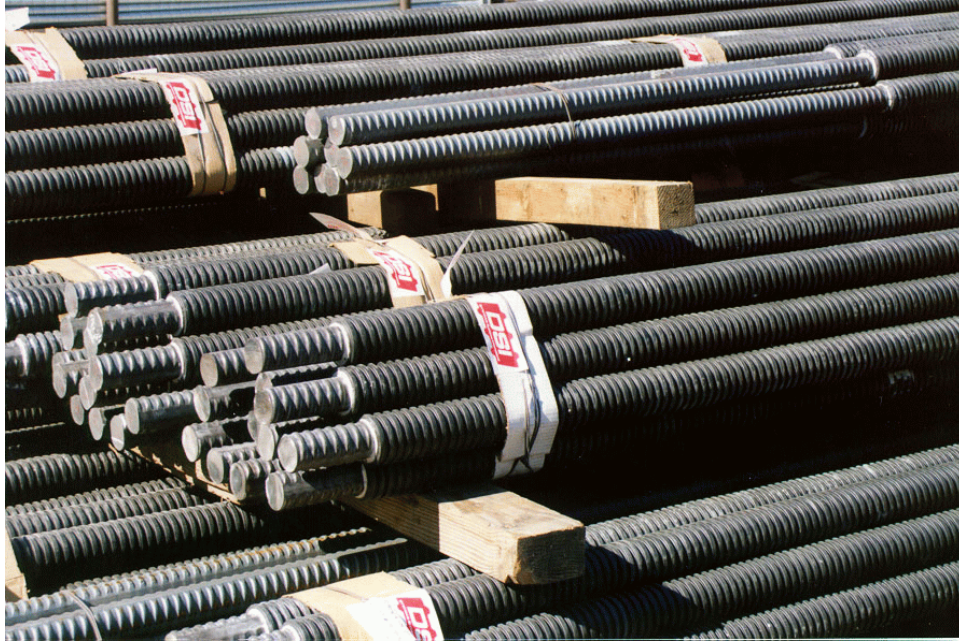
Photograph 8 - 3. Double Corrosion Protected (Encapsulated) Reinforcing Steel
