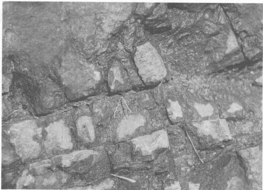
Figure 5.21 Weathered joint surface. Note the red colored clay between the rock surfaces.
