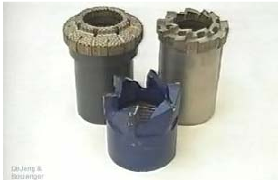
Figure 3-16. Coring bits: Diamond (top left), Carbide (top right), and Sawtooth (bottom center) (FHWA, 2002b).
