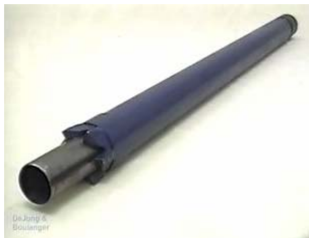
Figure 3-12. Pitcher sampler (FHWA, 1997, 2002b).
