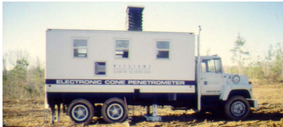
Figure 3-29. Cone penetration testing from cone truck.
