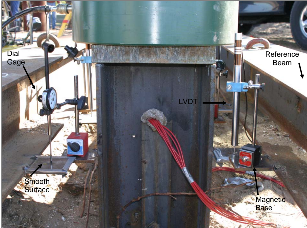
Figure 9-65. Load test movement monitoring components (FHWA, 2006a).
