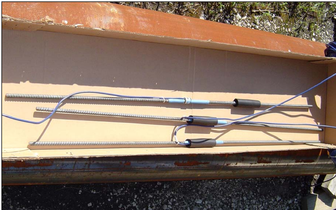
Figure 9-70. Sister bar vibrating wire gages for concrete embedment (FHWA, 2006a).
