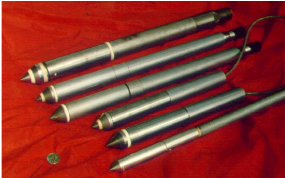
Figure 3-28. Cone and piezocone penetrometers (note the quarter for scale) (FHWA, 2002b).
