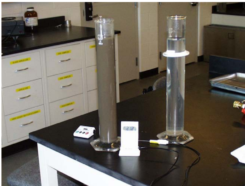
Figure 5-6. Soil hydrometer apparatus ( http://www.ce.siu.edu/ ).
