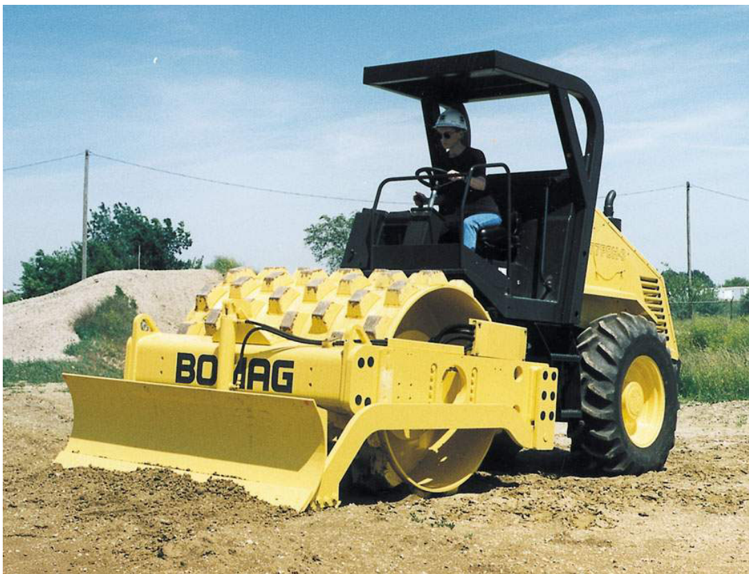
Figure 8-13. Sheepfoot roller ( photo courtesy of Bomag ).
