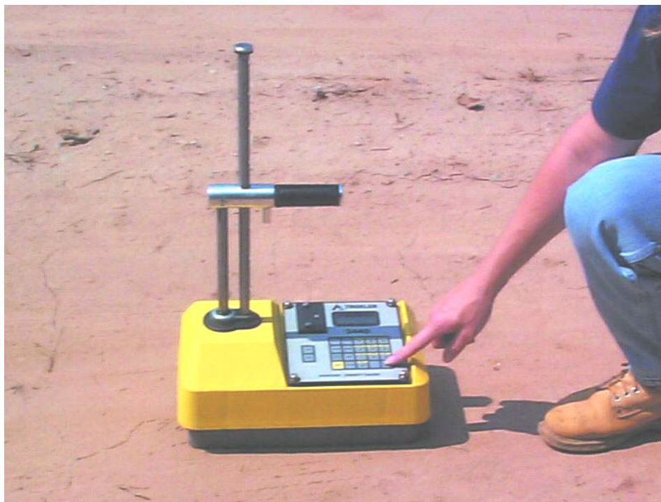
Figure 8-1. Nuclear densometer ( photo courtesy of Troxler ).
