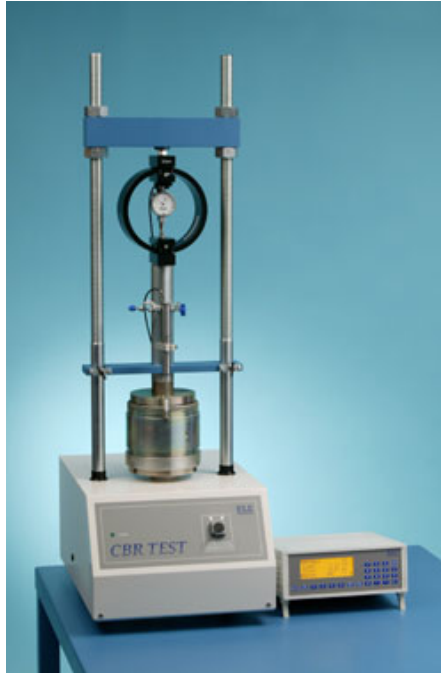
Figure 5-12. California Bearing Ratio test device ( http://www.ele.com/geot/cali.htm ).
