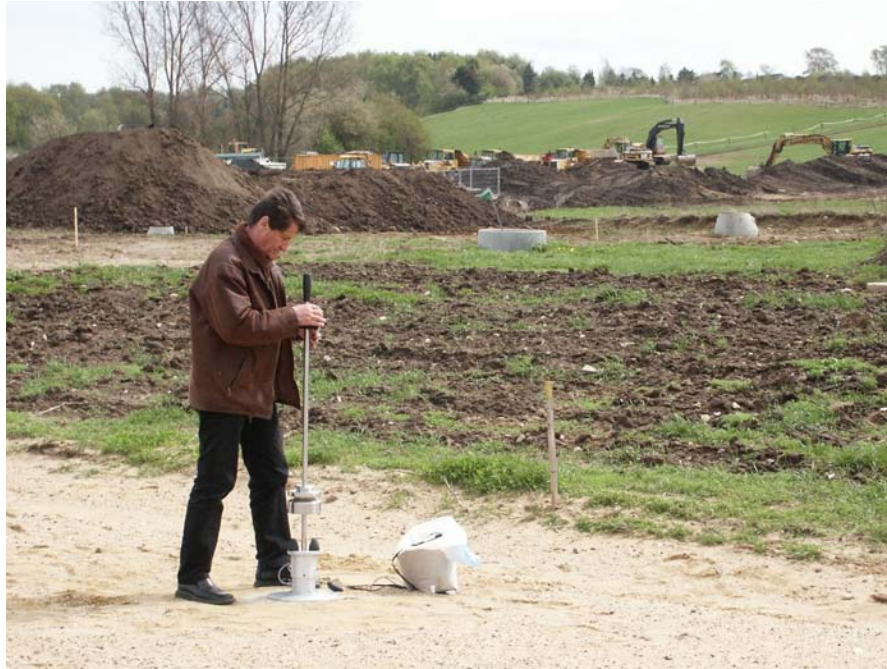
Figure 8-3. Lightweight deflectometer ( photo courtesy of Dynatest ).
