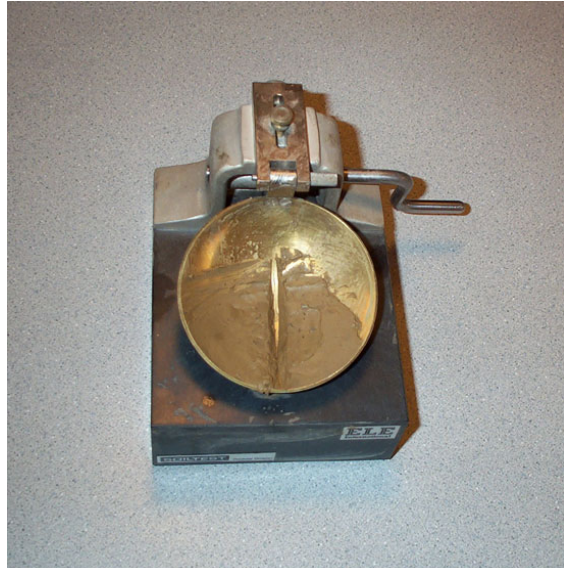
Figure 5-9. Liquid limit test device.
