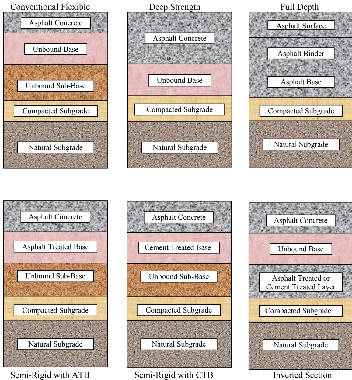
Figure 1-3. Some common variations of flexible pavement sections (NCHRP 1-37A, 2002).
