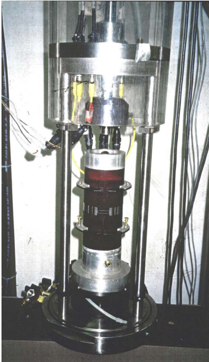
Figure 5-16. Triaxial cell set-up for resilient modulus test.
