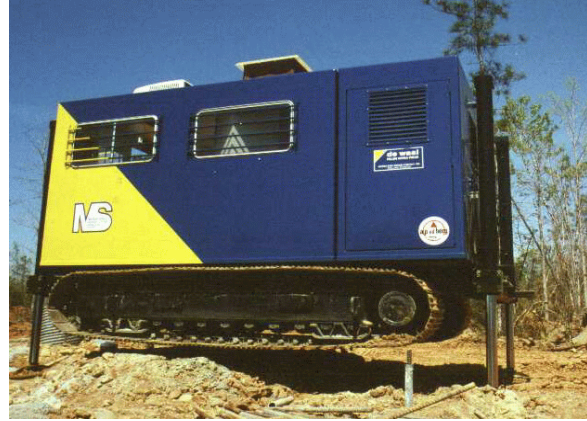
Figure 5-2. Direct-Push Technology: (a) Truck-Mounted and (b) Track-Mounted Cone Rigs.
