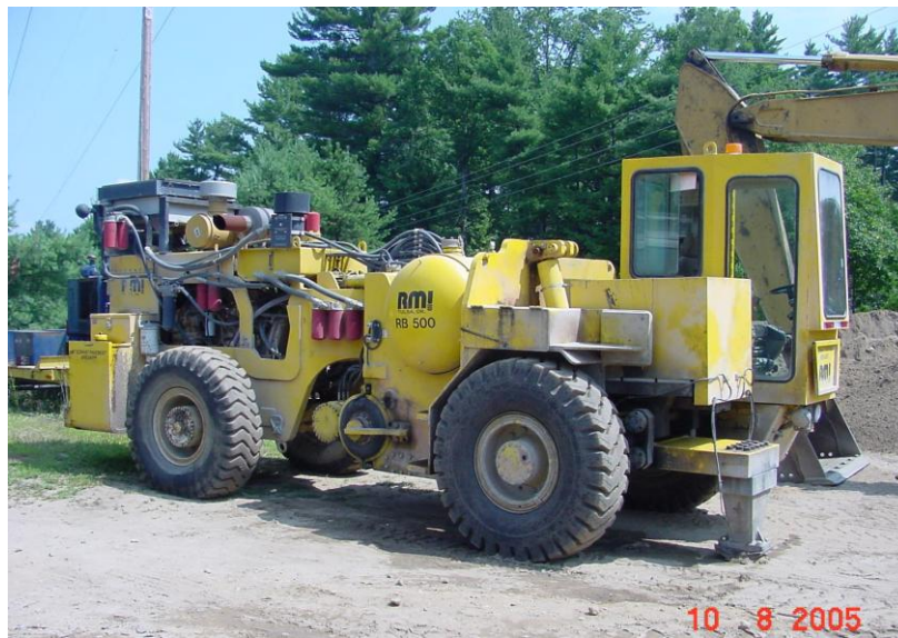
Figure 5 - Pavement breaker for rubblizing concrete
