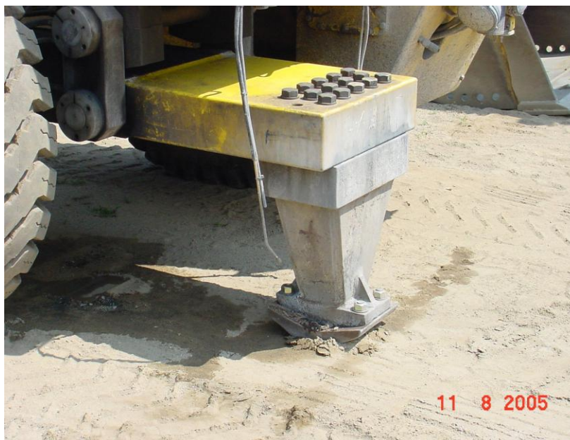
Figure 6 - Vibrating foot on pavement breaker
