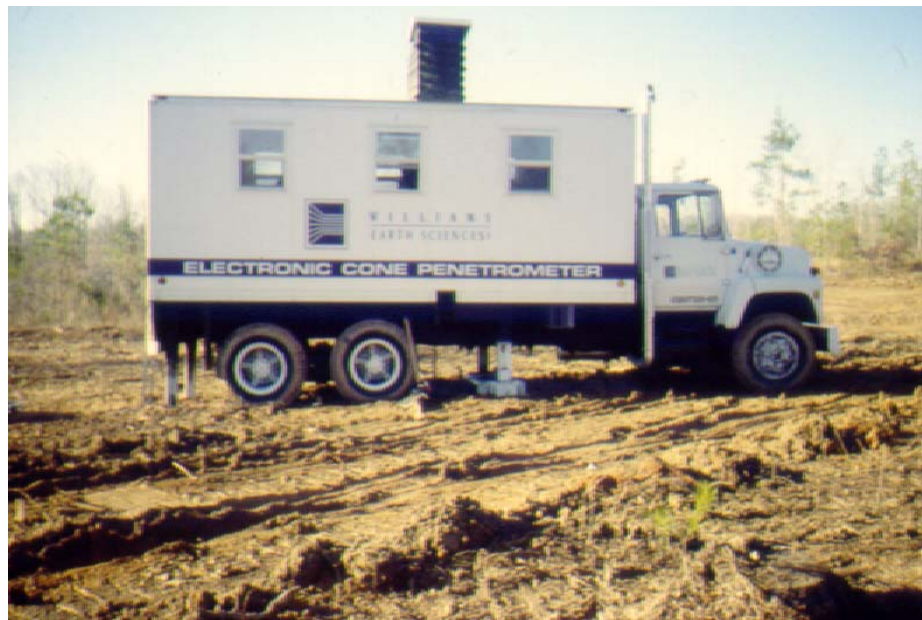
Figure 13. Cone penetration testing from cone truck.
