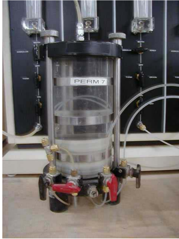
Figure 32. Flexible wall permeameter (photograph courtesy of GeoTesting Express).
