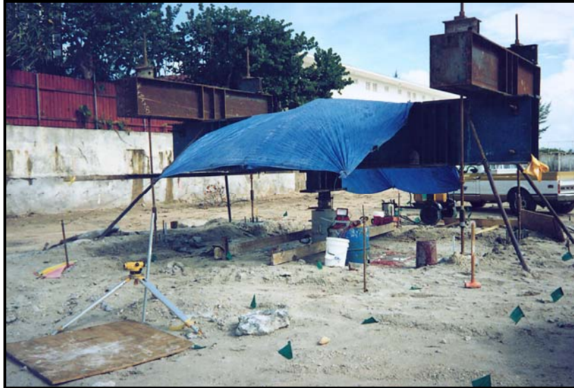
Figure 7.15: Static Load Test Setup on CFA Piles
