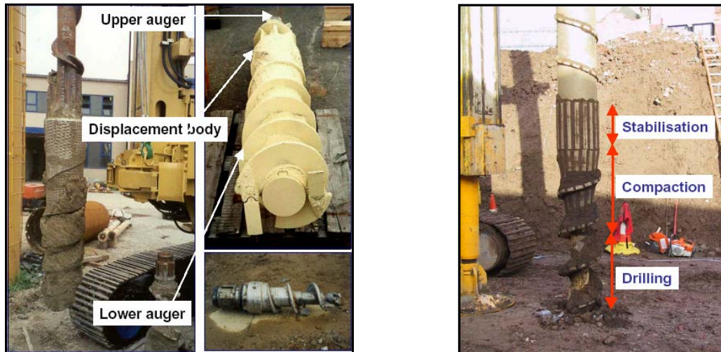
(a) Full Displacement Augers
