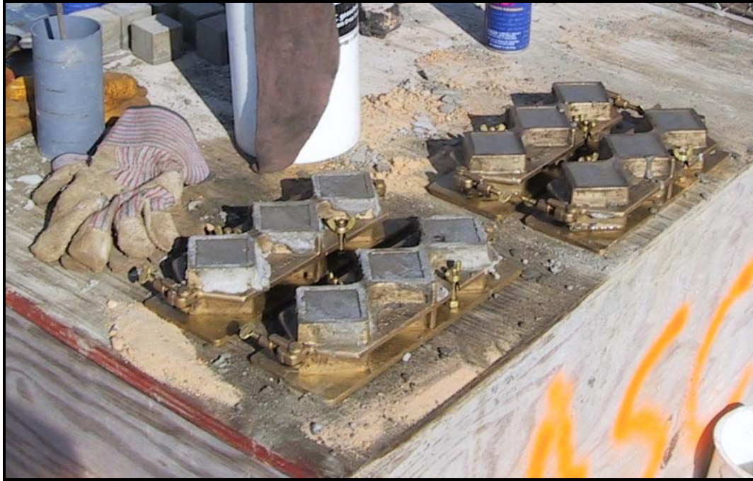
Figure 7.10: Cubes for Grout Testing
