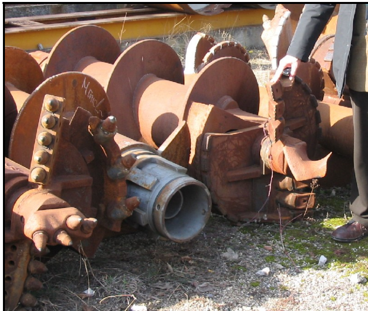
Figure 4.9: Cutter Heads for Hard Material (left) and Soil (right)
