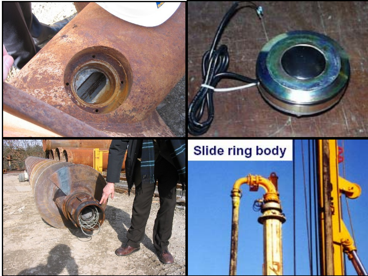
Figure 4.21: Sensor for Concrete Pressure at Auger Tip
