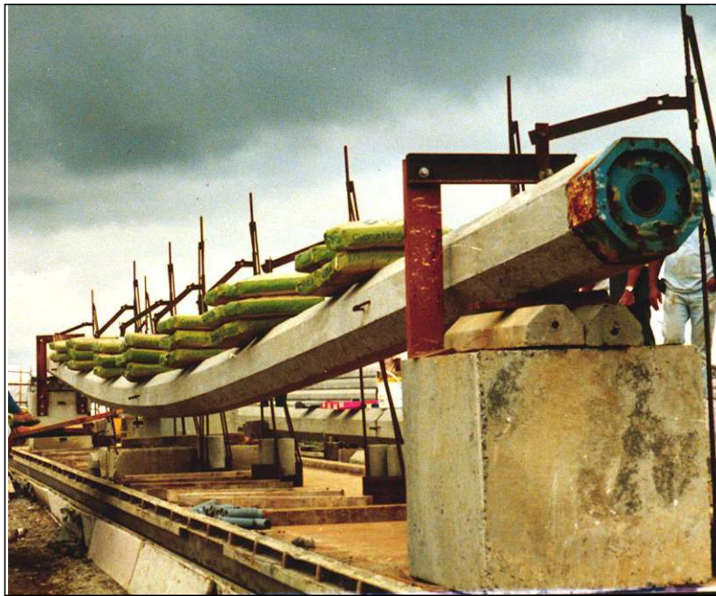
Fig. 7.40 Verifying the principle of the curvature probe
