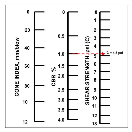
Figure 4. Relationship between cone index, CBR, and shear strength (C).
