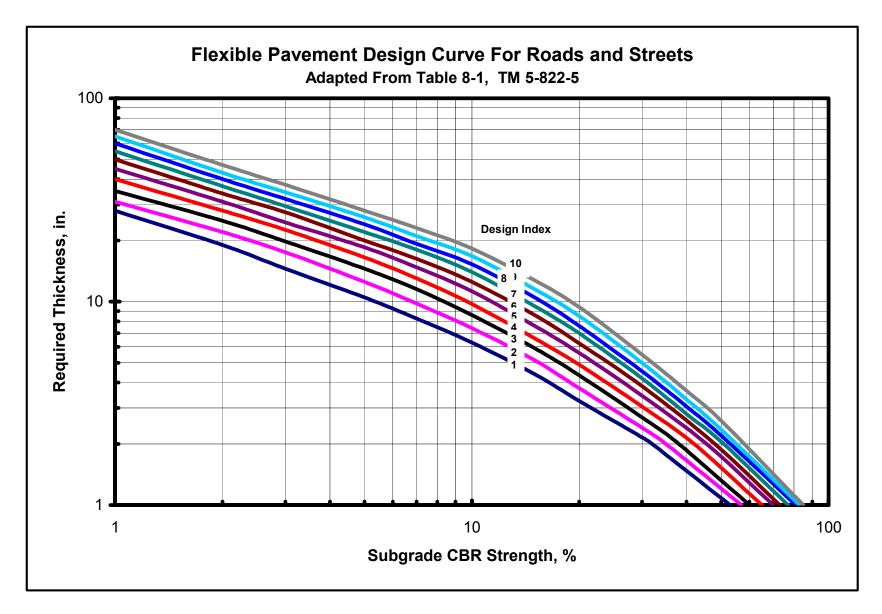
Figure 9. Flexible pavement design curves for roads and streets (adapted from Table 8-1 of TM 5-822-5).
