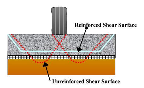
Figure 2. Improved bearing capacity reinforcement mechanism.
