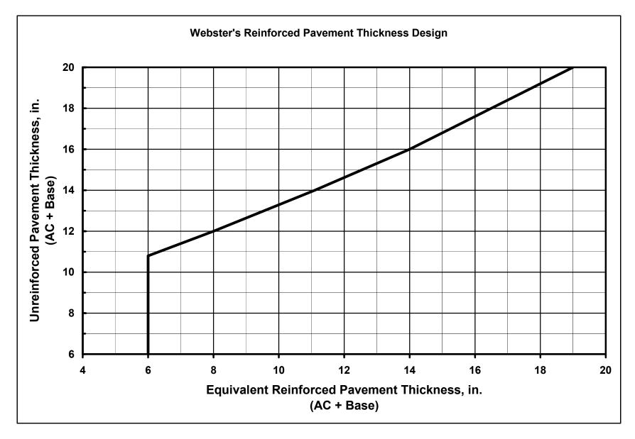
Figure 8. Webster's reinforced pavement thickness equivalency chart.
