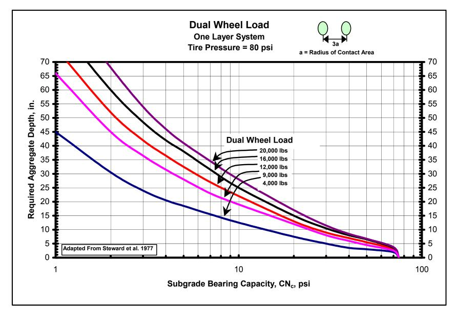
Figure 6. Aggregate-surfaced pavement design curves for dual-wheel loads.
