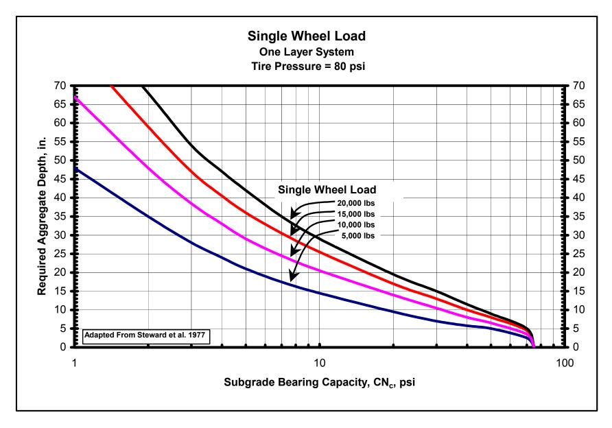
Figure 5. Aggregate-surfaced pavement design curves for single-wheel loads.
