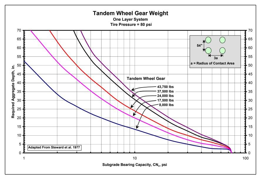
Figure 7. Aggregate-surfaced pavement design curves for tandem-wheel gear loads.
