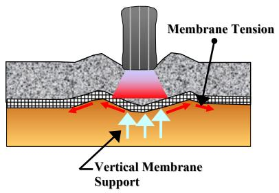
Figure 3. Tensioned membrane effect reinforcement mechanism.
