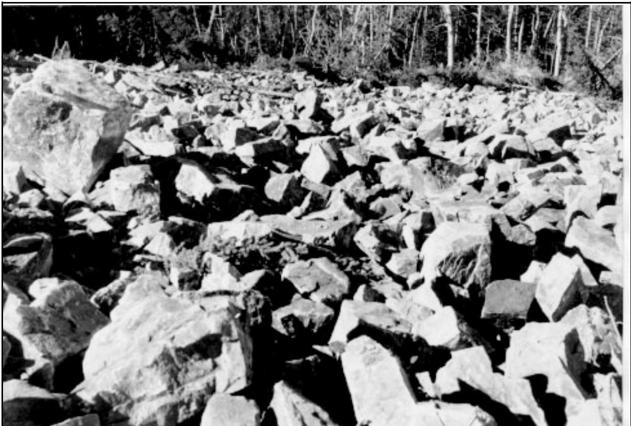
Figure 2-15.—Results of a major blast in a riprap quarry.
