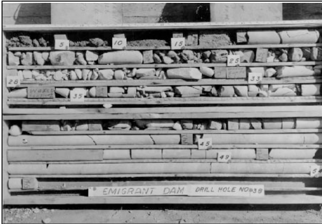
Figure 2-49.—Arrangement of cores in a core box to ensure proper identification of samples.
