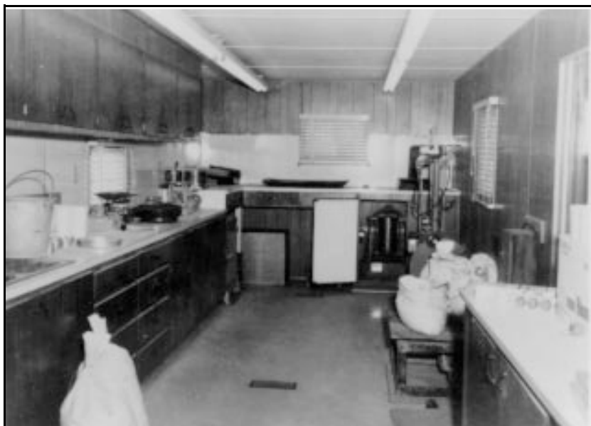
a. Semimobile trailer unit used as a field laboratory.
