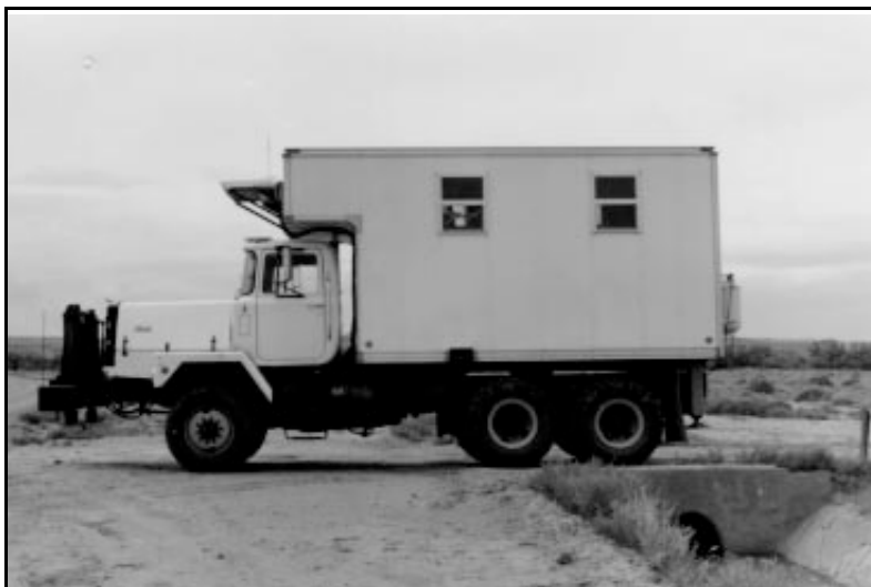
Figure 2-54.—Electronic cone penetrometer testing vehicle.
