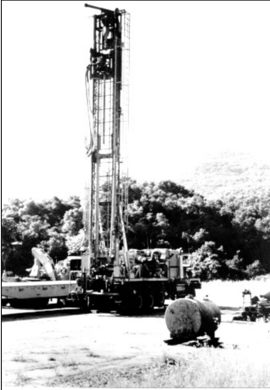
Figure 2-29.—Top-head drive drill with head-in mast for drilling.
