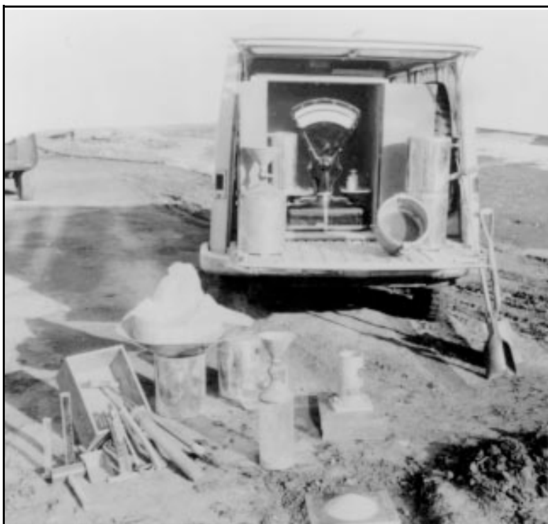
b. Type V laboratory—vehicle equipped for on-site earthwork control tests.
