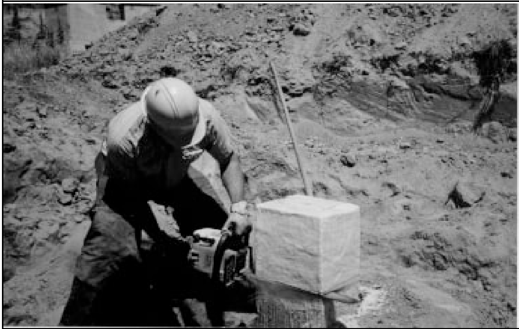
Figure 2-40.—Chain saw equipped with carbide-tipped blade being used to cut block sample.
