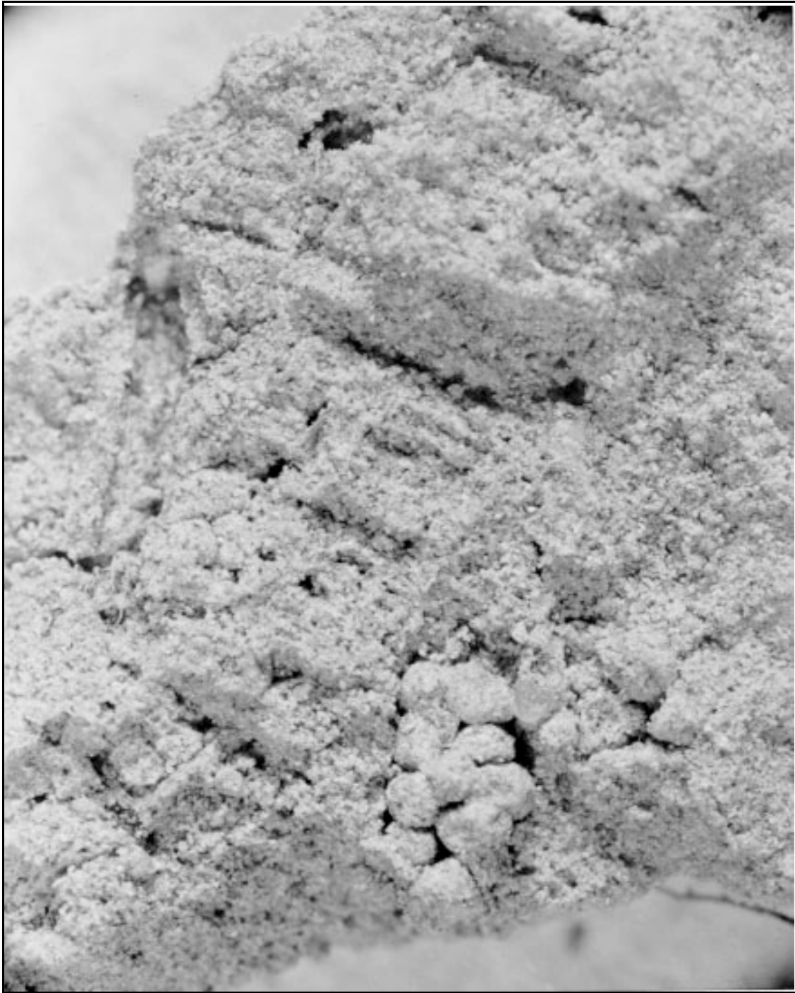
Figure 2-8.—Photomicrograph showing typical open structure of silty loess.
