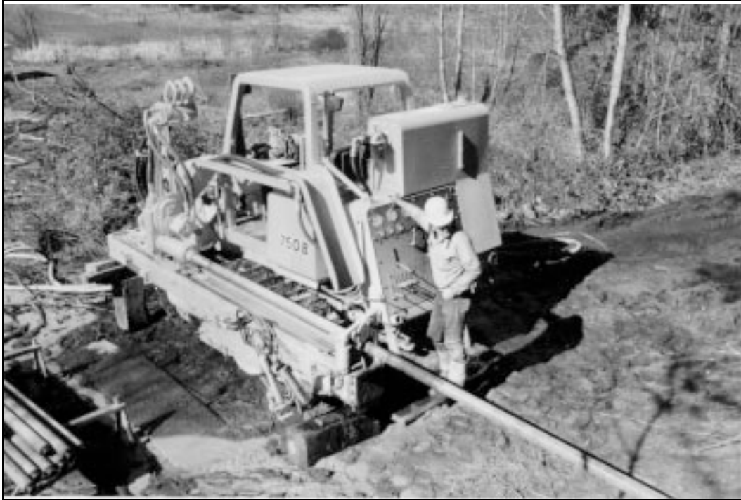
Figure 2-33.—Horizontal rotary drill. Aardvark model 500 drill with adjustable box-beam slide, crawler-tractor mounted.
