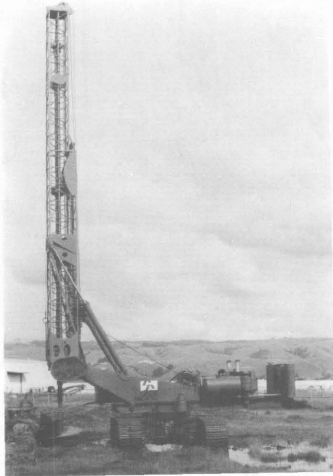
Figure 4.3. A typical crawler-mounted drilling machine (Courtesy of Case Pacific Company)
