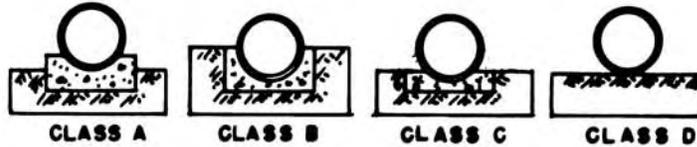
CLASS A- CONCRETE CRADLE; B- COMPACTED GRANULAR MATERIAL; C- COMPACTED GRANULAR MATERIAL OR DENSELY COMPACTED BACKFILL; D- FLAT SUBGRADE.
