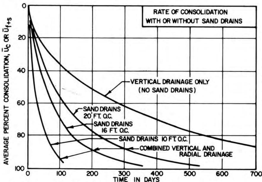
TO STUDY VARIOUS SPACING OF DRAINS, VALUES OF  $\bar{U}_c$  VS TIME ARE COMPUTED FOR  $d_e = 10', 16' \text{ \& } 20'$ . RESULTS ARE PLOTTED AT LEFT.
