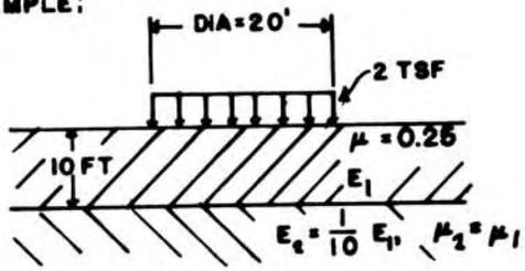
I. DETERMINE PROFILE OF STRESS INCREASE DUE TO APPLIED LOAD BELOW THE EDGES.
