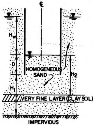
IF THE TOP OF FINE LAYER IS AT A DEPTH GREATER THAN WIDTH OF EXCAVATION BELOW CUT OFF WALL BOTTOM, SAFETY FACTORS OF FIGURE 2 APPLY, ASSUMING IMPERVIOUS BASE AT TOP OF FINE LAYER.
