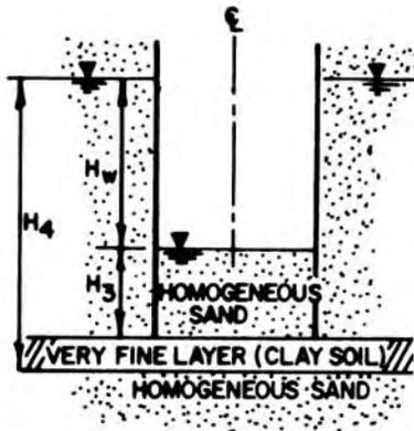
TO AVOID BOTTOM HEAVE,  $\gamma_T \times H_3$  SHOULD BE GREATER THAN  $\gamma_W \times H_4$ .
