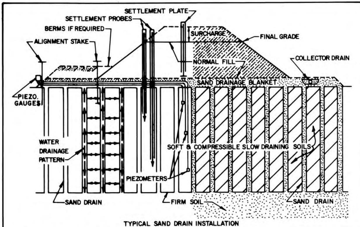
**DIAMETER OF DRAINS** RANGES FROM 6 TO 30 IN., GENERALLY BETWEEN 16 AND 20 IN.
