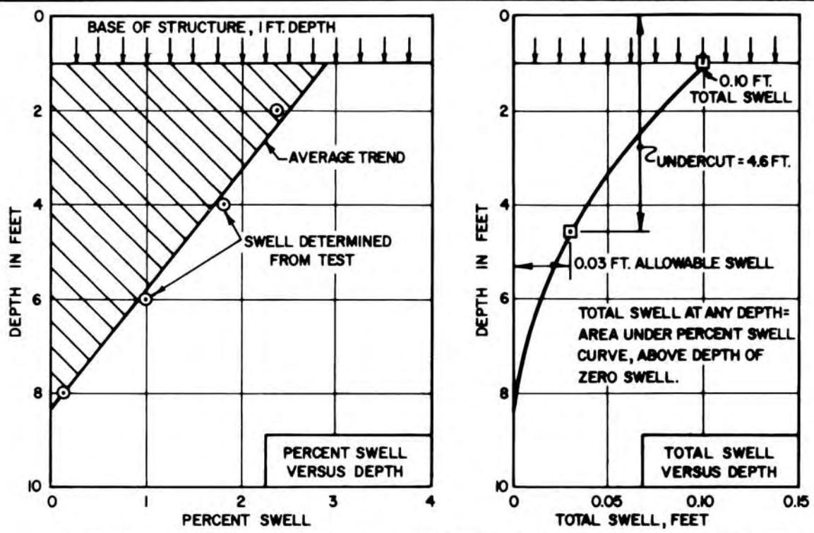
MATERIALS INVESTIGATED ARE CLAYS, HIGHLY OVERCONSOLIDATED BY CAPILLARY STRESSES THAT ARE EFFECTIVE PRIOR TO THE CONSTRUCTION OF THE STRUCTURE UPON THEM.
