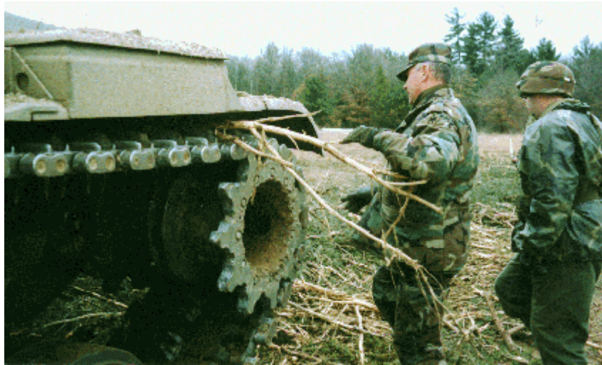
Figure 12. Tree slash caught in tracks during cornering.
