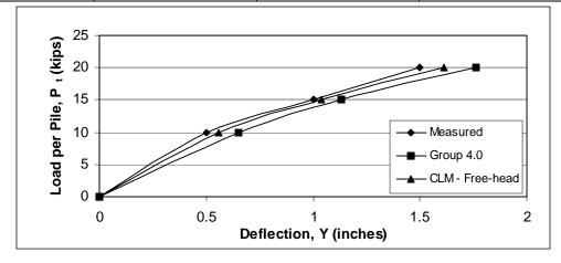
Figure 5 – Pile Group Comparison (load test data from Brown et al., 1988)
