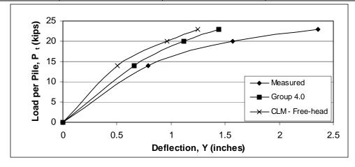
Figure 8 – Pile Group Comparison (load test data from Rollins et al., 1998)
