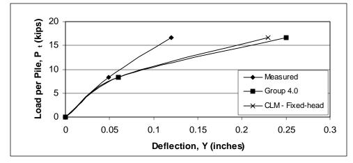
Figure 6 – Pile Group Comparison (load test data from Kim et al., 1979)
