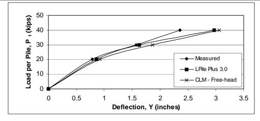
Figure 4 – Single Pile Comparison (load test data from Rollins et al., 1998)
