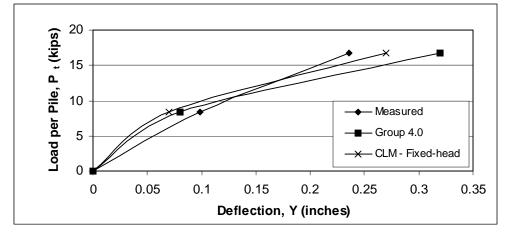
Figure 7 – Pile Group Comparison (load test data from Kim et al., 1979)
