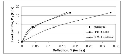
Figure 3 – Single Pile Comparison (load test data from Kim et al., 1979)
