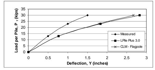
Figure 2 – Single Pile Comparison (load test data from Brown et al., 1988)
