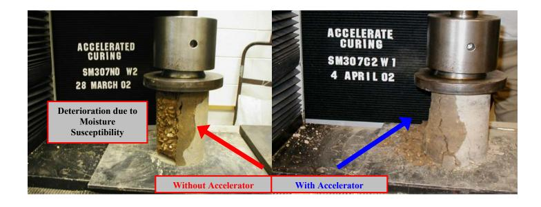
FIGURE 1 Moisture susceptibility of SM sample stabilized with 2.5 percent Silicate 1
