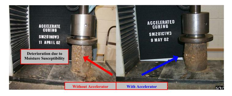
FIGURE 2 Moisture susceptibility of SM sample stabilized with 1 percent Polymer 6
