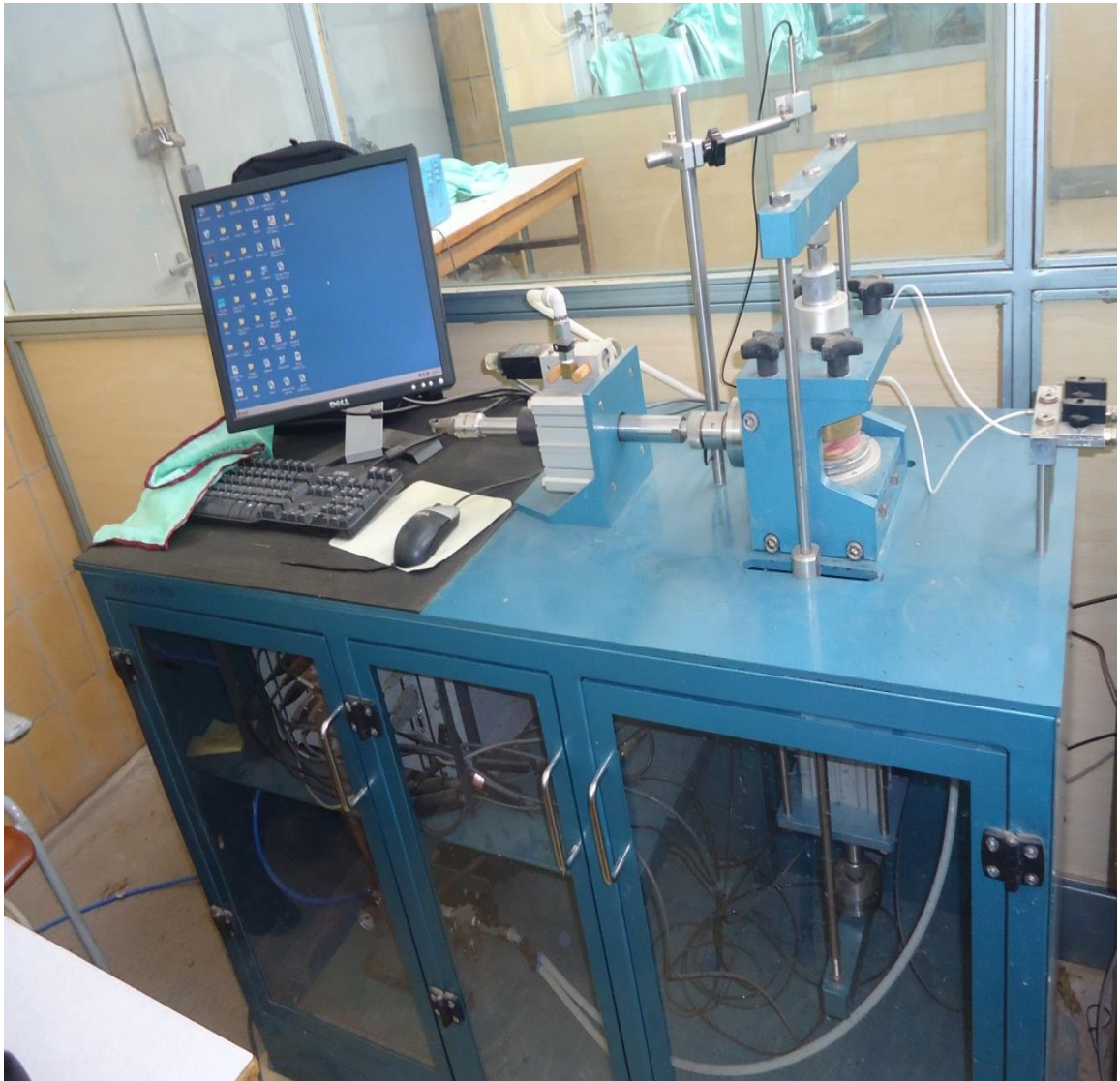
Fig 3.3 Cyclic shear apparatus and its general features
